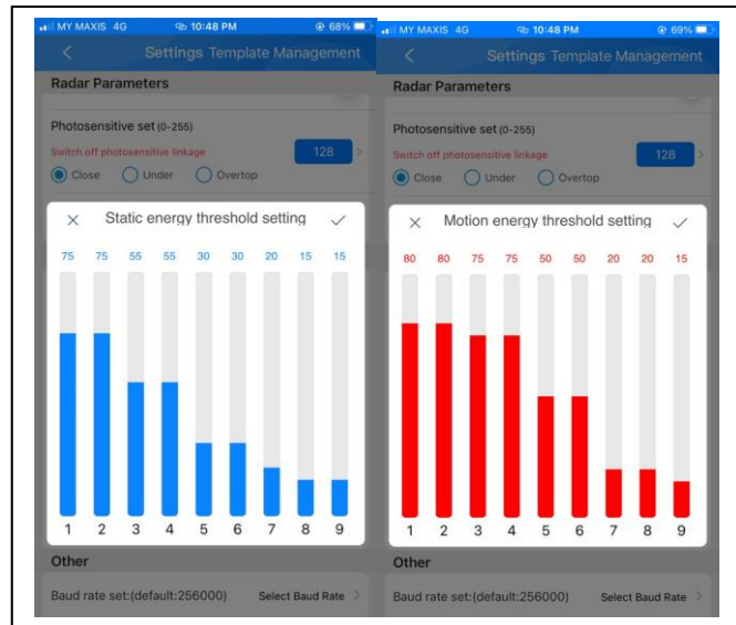
Figure 3.15: Static and Motion Energy Threshold Calibration
