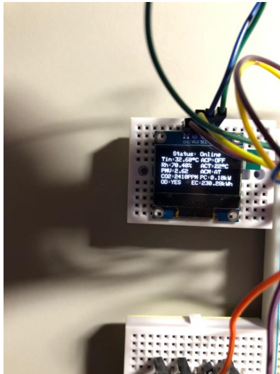
Figure 3.13: OLED display of Smart AC Controller
