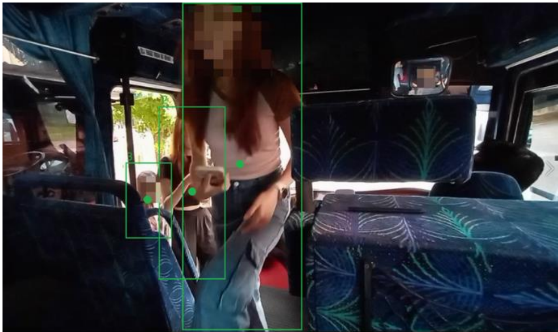
Figure 4-6 Passenger detection when getting on bus part 2
