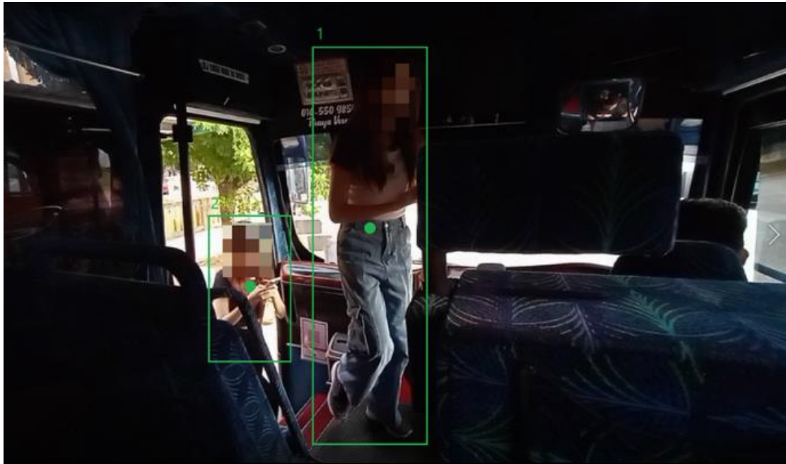
Figure 4-5 Passenger detection when getting on bus part 1
