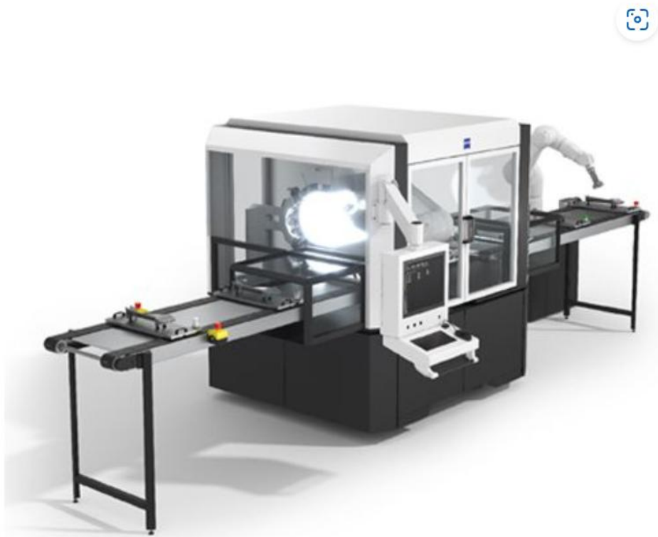
Figure 2.1.1 Non-contact automated surface detection machine
