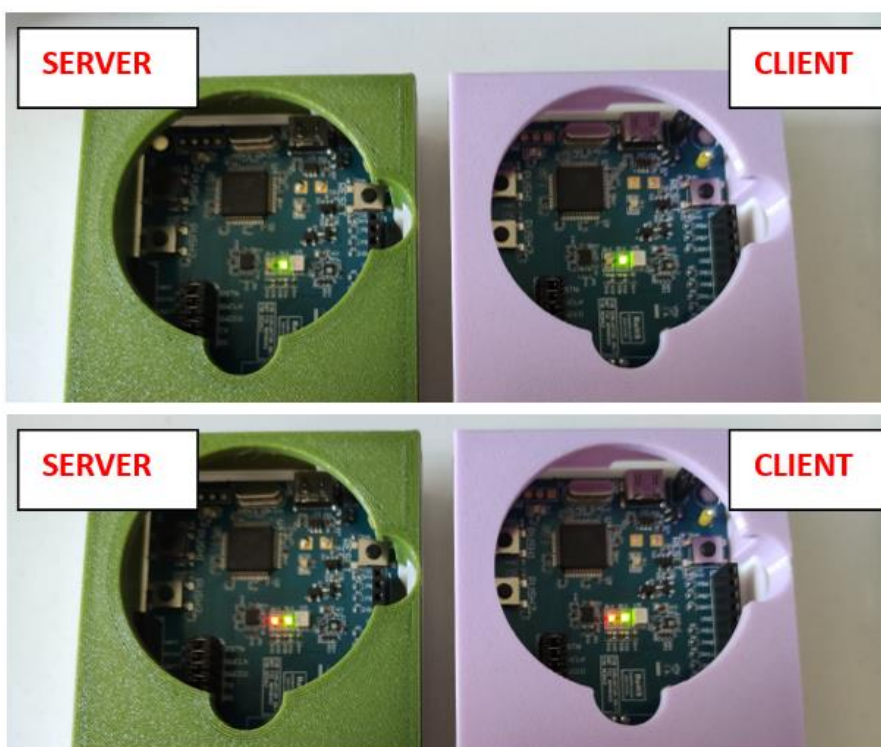
Figure 3.10: Binking LED3 indicates boards are communicating.
