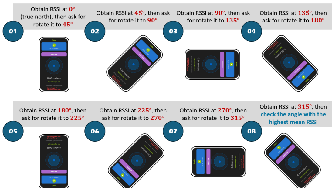
Figure 3.55: Operation in rotating the mobile device to estimate the direction.
