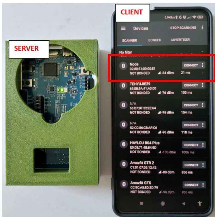
Figure 3.12: Evaluation board (Node) is discovered in the application.
