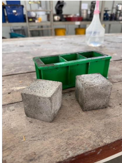
Figure 3.5 Mortar cube (50mm x 50mm x50mm)
