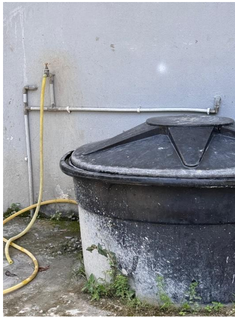
Figure 3.6 Water tank for curing
