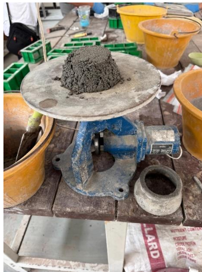
Figure 3.8 Flow table test
