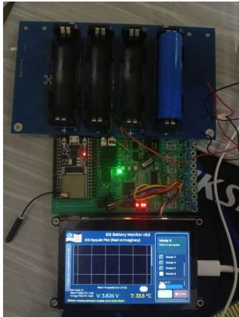
Figure 5.1 : Hardware Setup. Battery fixture, ESP32-S3 interface board with DNB110xA, and JC4827W543 display showing the LVGL “EIS Battery Monitor” screen
