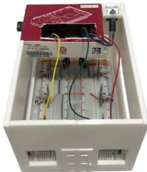
Figure 5.5 The enclosure designed for the hardware components using Tinkercad
