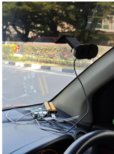
Figure 5.1 Hardware setup of the fatigue detection system inside the vehicle.
