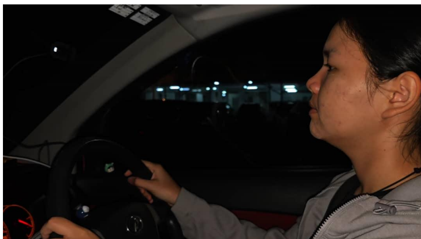
Figure 6.1(b) shows the system setup during night-time driving, where the system relied on cabin lighting to detect facial features in low-light conditions.
