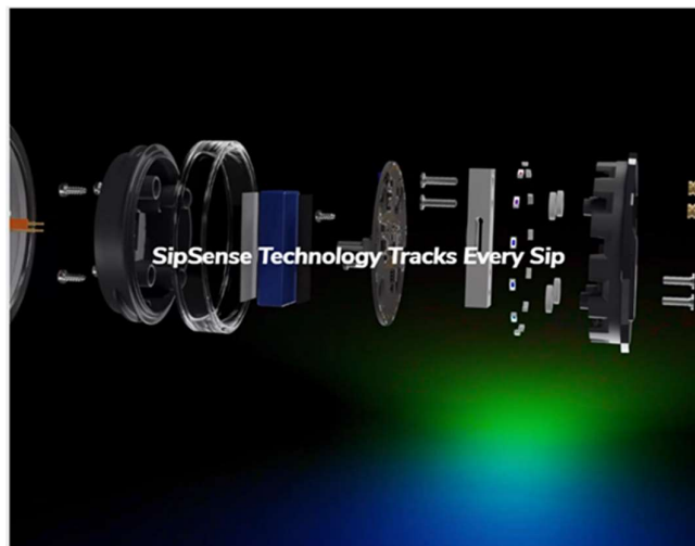
Figure 2.2.1 Exploded view of HidrateSpark Pro SipSense technology sensor module
