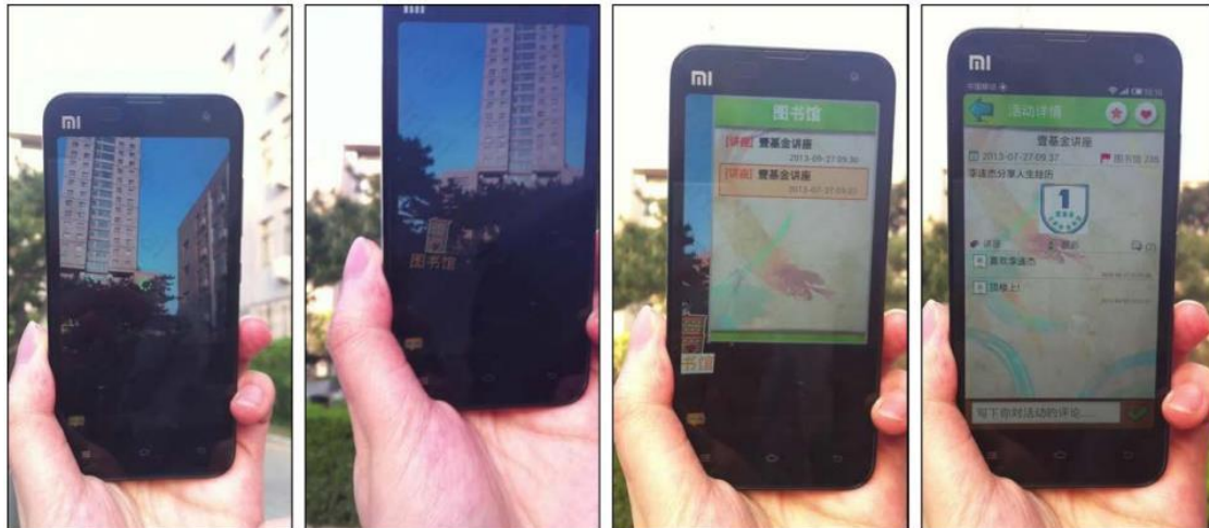
Figure 2.1.1.2: AR and GPS based activity information module for Mobile Campus Touring System. [2]
