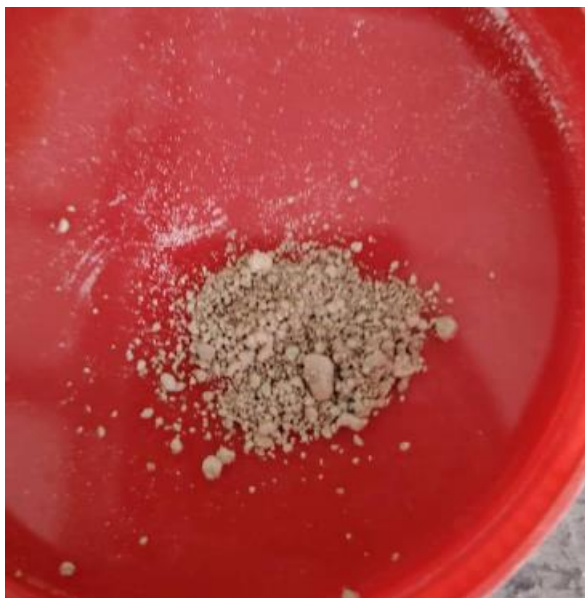
Figure 3.5: Sieved and Oven-dried Alum Sludge.
