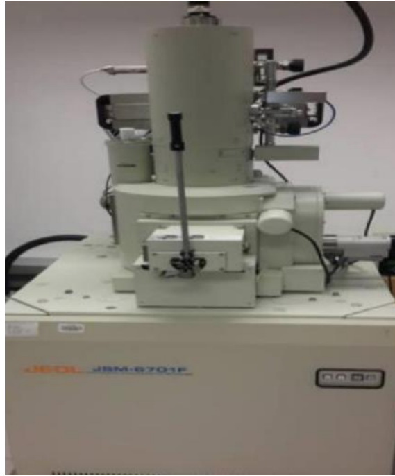
Figure 3.17: Machine Used to Conduct Scanning Electron Microscopy (SEM) Analysis.
