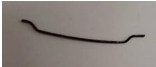
Figure 3.10: Hooked Shape Steel Fibre.
