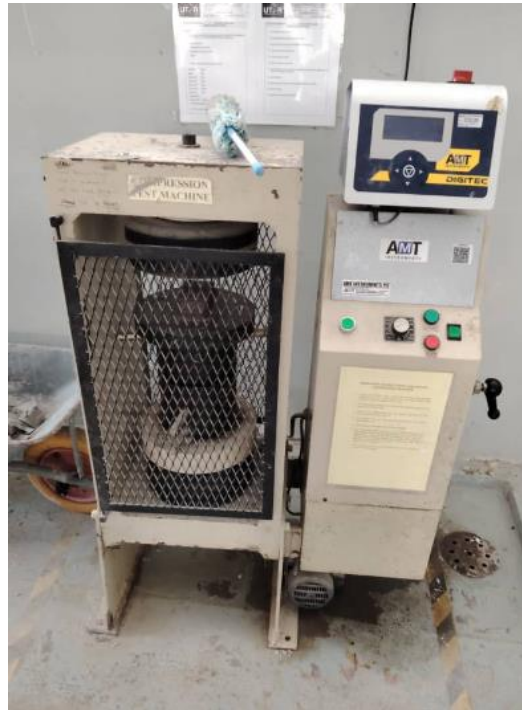
Figure 3.16: Compression Machine for Compression Test.
