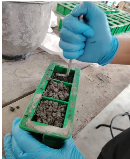
Figure 3.12: Manual Compaction of Fresh Concrete Mixes.
