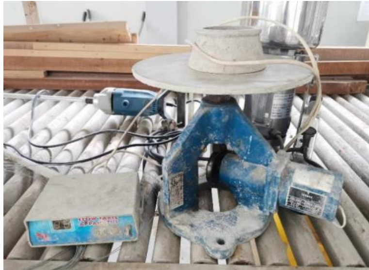
Figure 3.15: Flow Table Apparatus with Fully Filled Mould.
