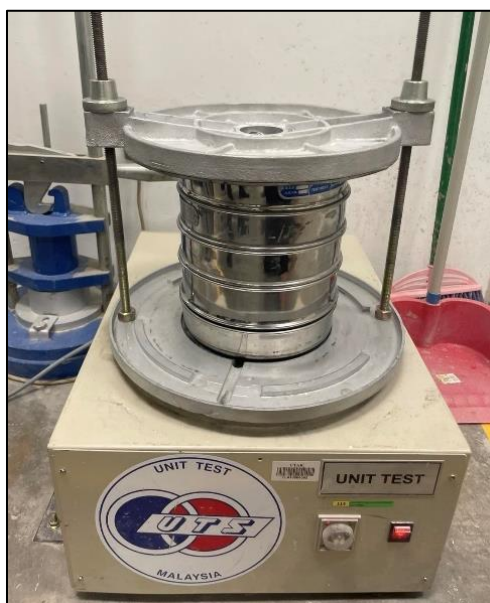
Figure 3.11: Set Up of Sieve Analysis Test for Coarse Aggregate.
