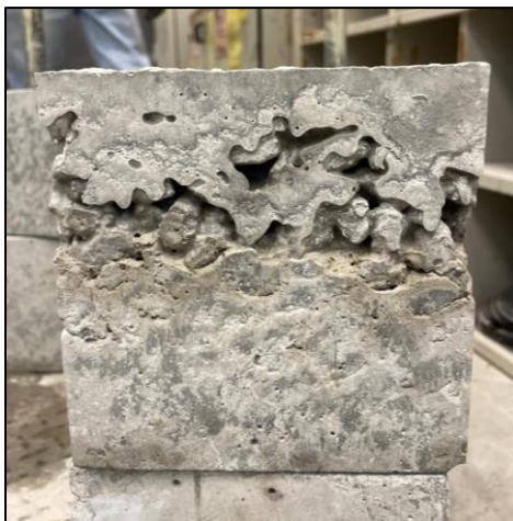
Figure 4.13: Observed Honeycombing in NC-0.25 Specimen.
