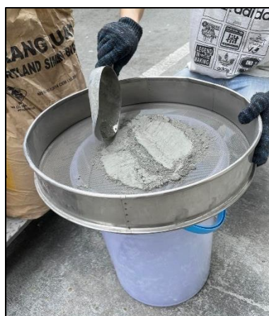
Figure 3.3: Sieving of Cement.
