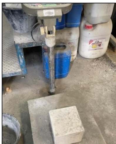
Figure 3.17: Weighing of Concrete using Digital Scale.
