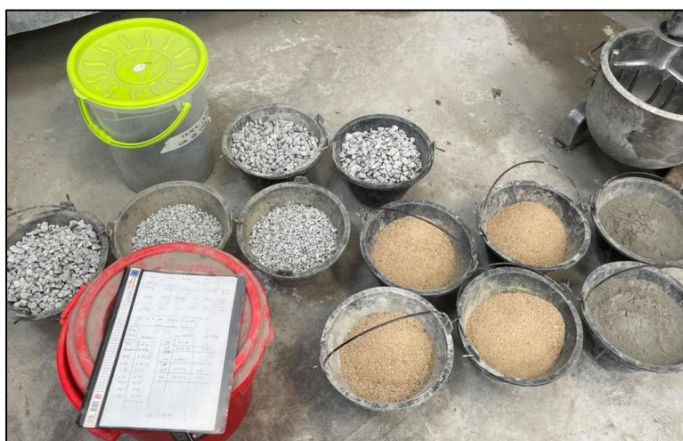
Figure 3.8: Weighted Materials Placed in Buckets.
