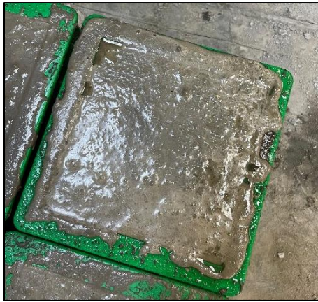
Figure 4.9: Bleeding Observed in the NC-0.30 mix.
