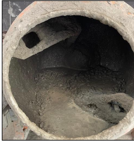
Figure 4.8: Segregation Observed in the NC-0.30 mix.
