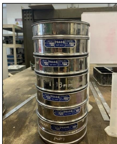
Figure 3.10: Set Up of Sieve Analysis Test for Fine Aggregate.
