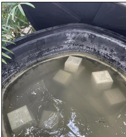
Figure 3.12: Water Curing for the Concrete Specimens.
