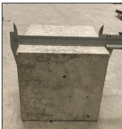
Figure 3.18: Measuring of Dimensions using Vernier Calliper.
