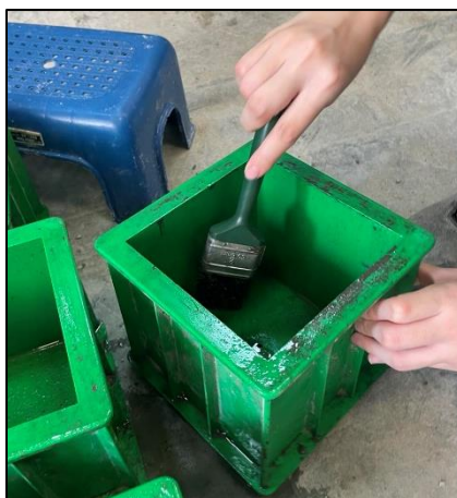
Figure 3.9: Oiling of Cube Moulds.
