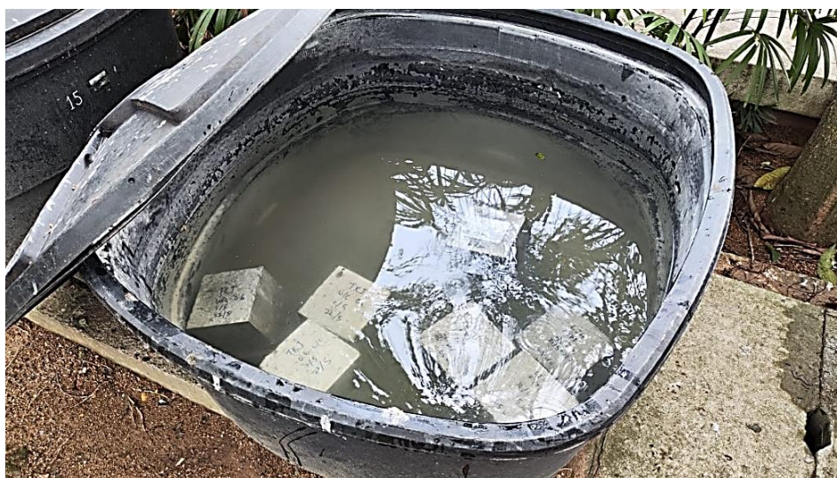
Figure 3.13: Water Curing Process for the Concrete Specimens.
