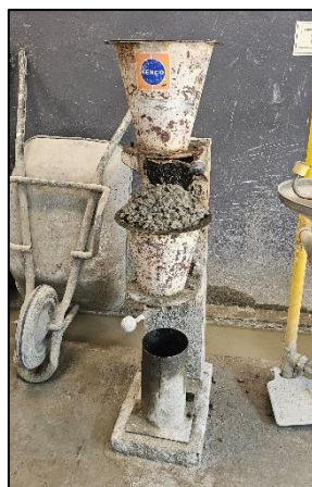
Figure 3.17: Compacting Factor Test Apparatus.
