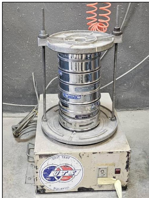
Figure 3.12: Sieve Analysis Setup for Fine Aggregate.
