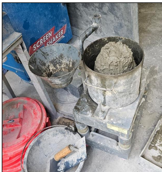
Figure 3.16: Slumped Concrete in Cone Container.
