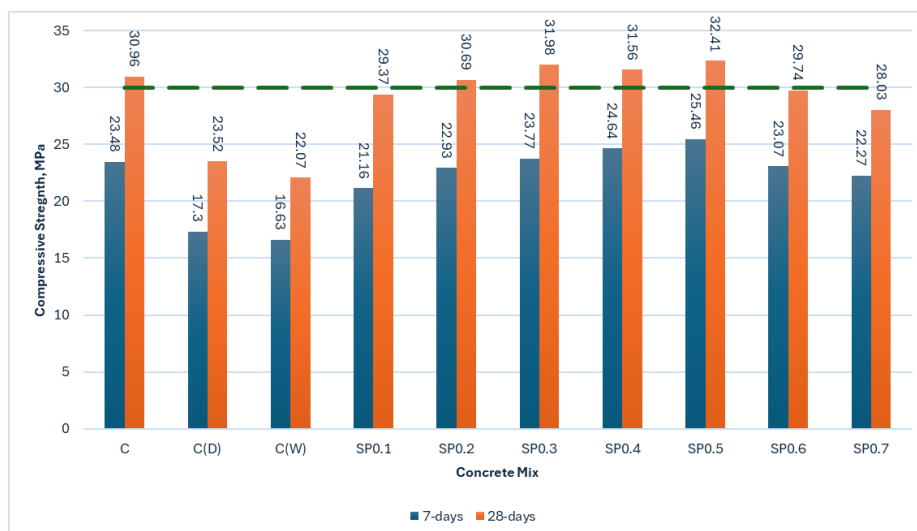
Figure 4.13: Graph of Compressive Strength against Concrete Mix.
