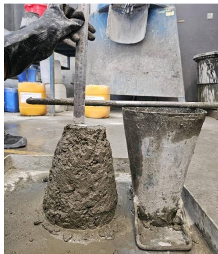
Figure 3.9: 50mm of Slump Was Measured.
