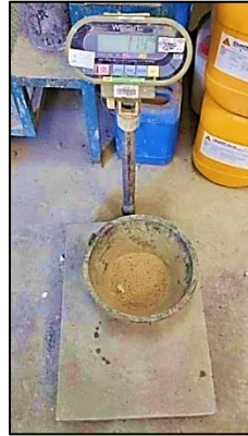
Figure 3.8: Fine Aggregate Was Weighted.
