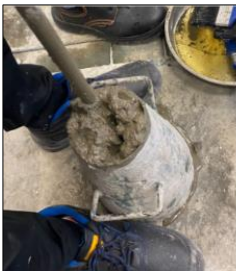
Figure 3.14: Concrete Mix Was Tamped Using Tamping Rod.
