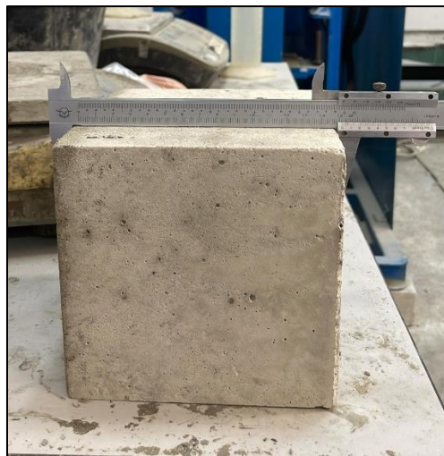
Figure 3.18: Dimension of Cube Specimen Was Measured by using Vernier Caliper
