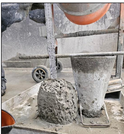
Figure 3.15: Slump Value Was Determined.
