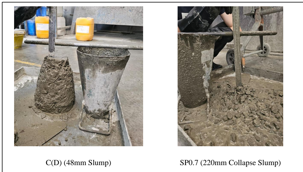
Figure 4.6: Slump Under Delayed Casting and Re-Dosing with 0.7% of SP.
