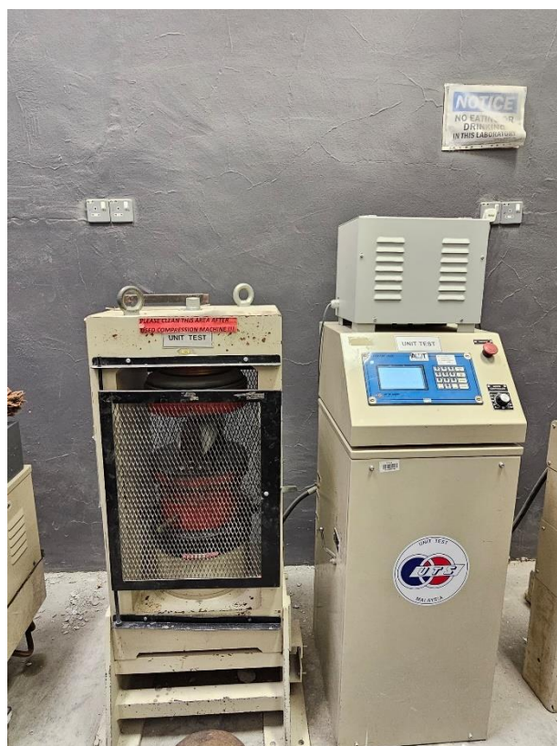
Figure 3.20: Splitting Tensile Test.
