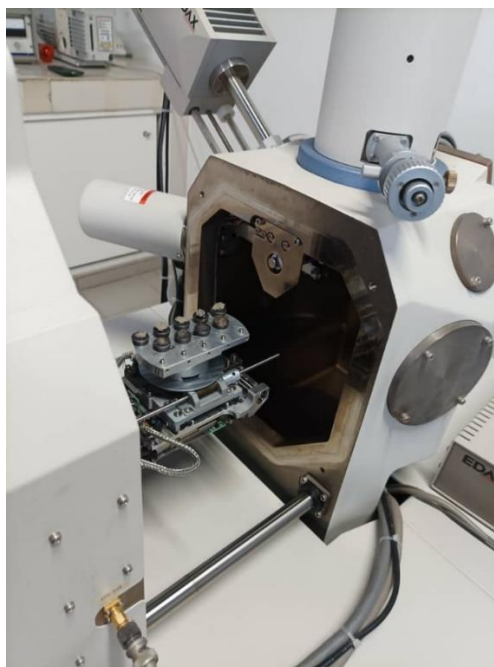
Figure 3.27: Specimen were Placed into Vacuum Chamber of SEM Machine.
