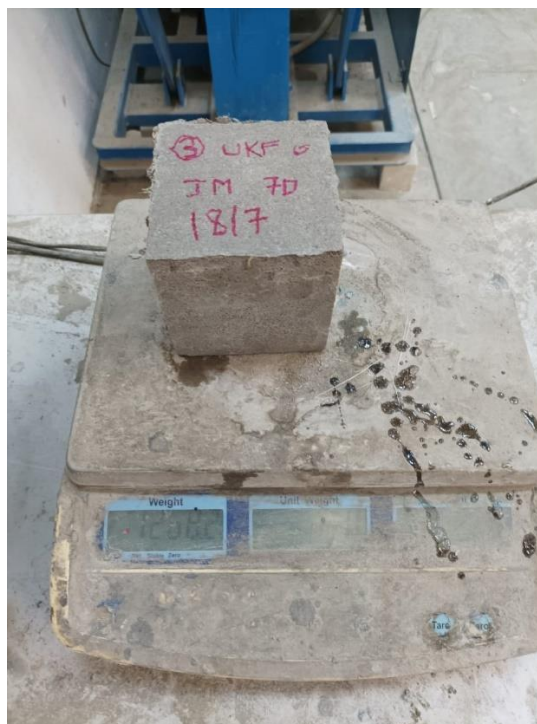
Figure 3.18: Concrete Weighed Using a Weighing Machine.
