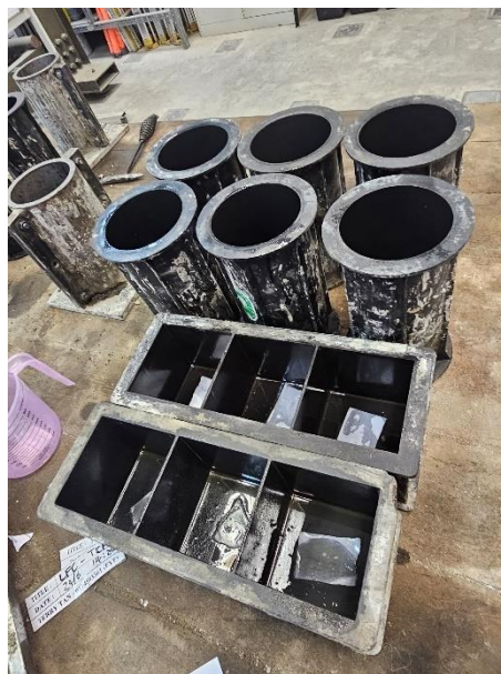
Figure 3.13: Oil Applied on Mould's Surface.
