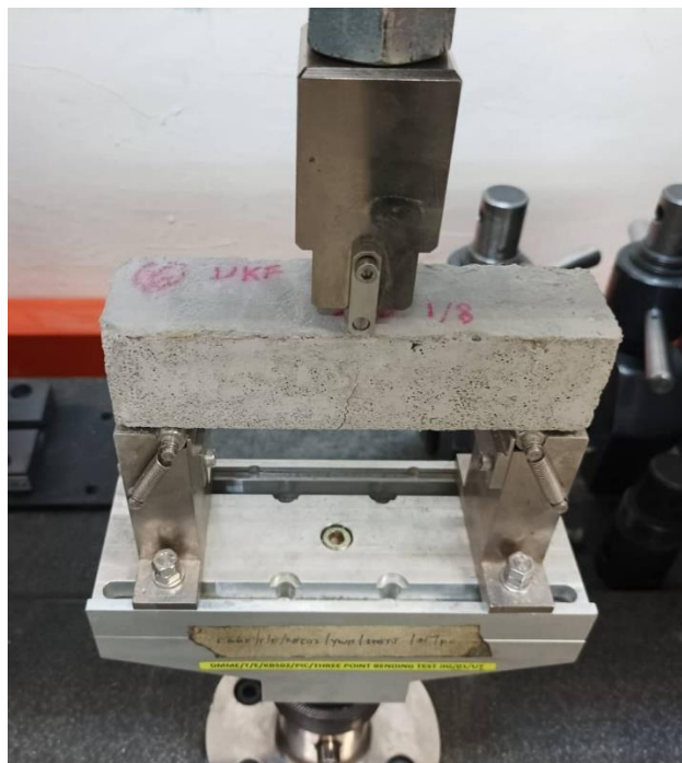
Figure 3.22: Setup of Specimen for Flexural Test.
