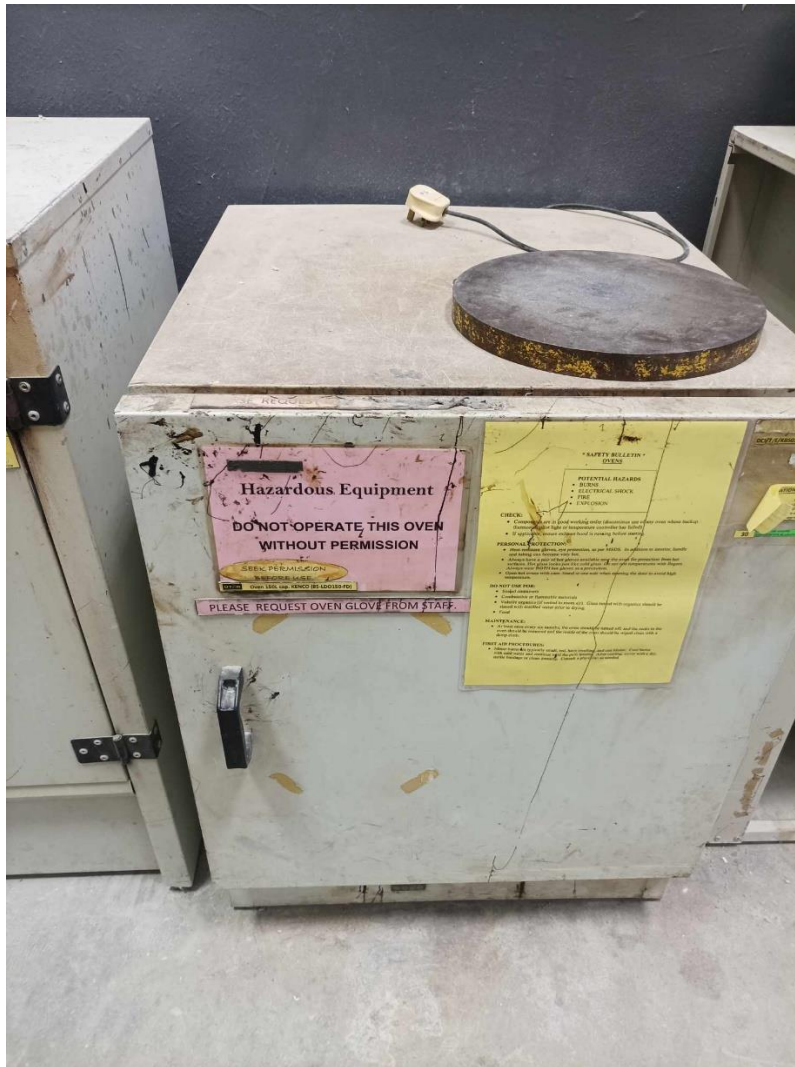
Figure 3.3: Oven for Dry Sand.
