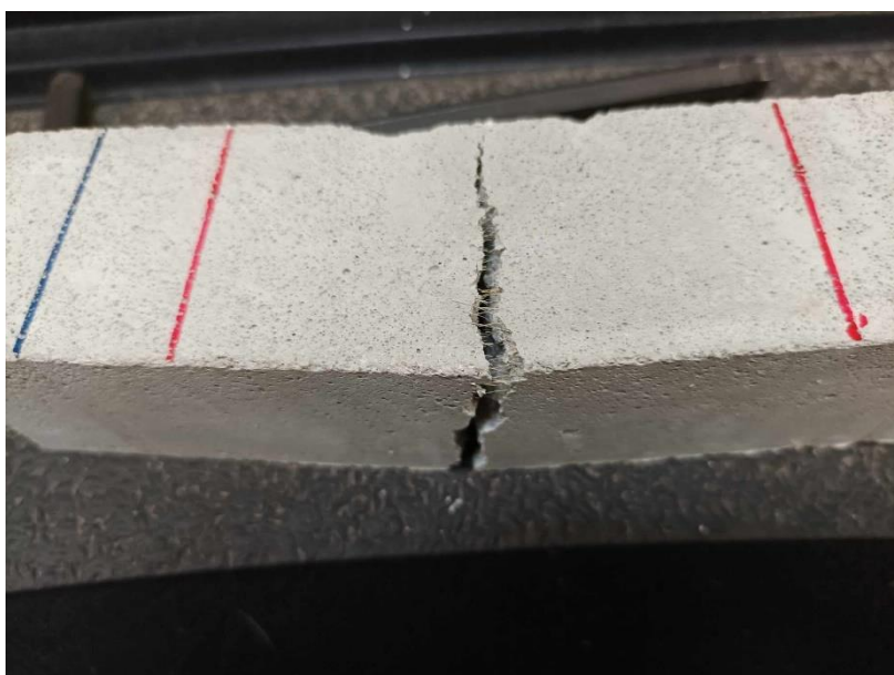
Figure 5.7: Failure of LFC-TF 12HR in Flexural Test.
