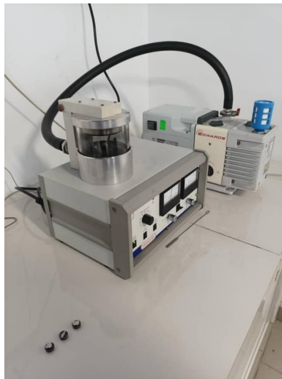
Figure 3.26: Sputter Coater Machine with Vacuum Pump (labelled "EDWARDS").
