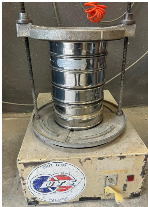
Figure 3.5: The Photo of Sieve Analysis Pan on Sieve Shaking Pan
