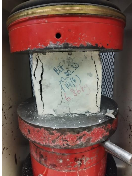
Figure 3.17: The Photo of Mortar Cube Crack in Compressive Strength Test
