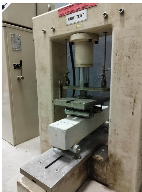
Figure 3.21: The Photo of Flexural Test
