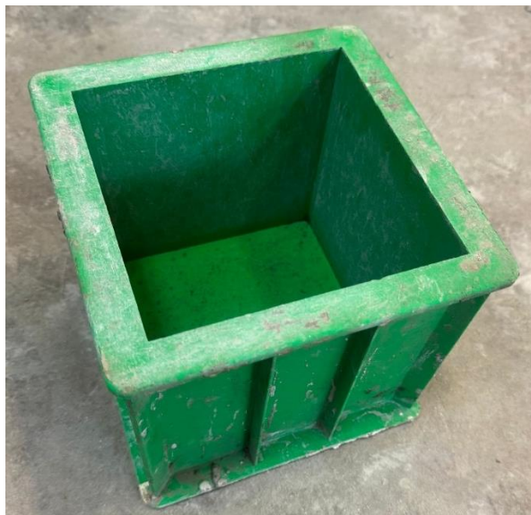
Figure 3.13: The Photo of Cube Mould
