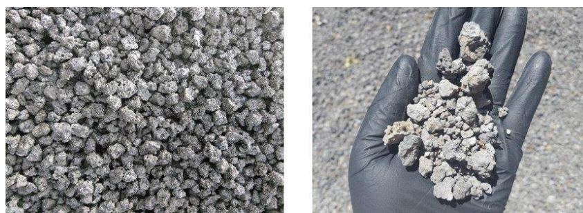
Figure 2.10: 0 – ¾ Inch Processed EAF Slag and A Variety of EAF Slag Sizes in a Gloved Hand for a reference. (US EPA, 2021)
