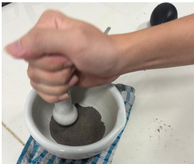
Figure 3.23: The Photo of the Apparatus Grinds the Sample into Powder.
