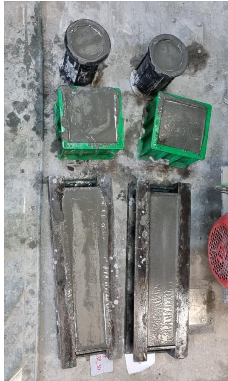
Figure 3.15: The Photo of Mortar Curing
