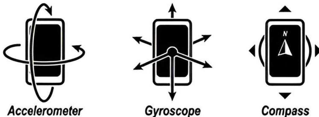
Figure 2.7 Smartphone as 3 PDR sensor
