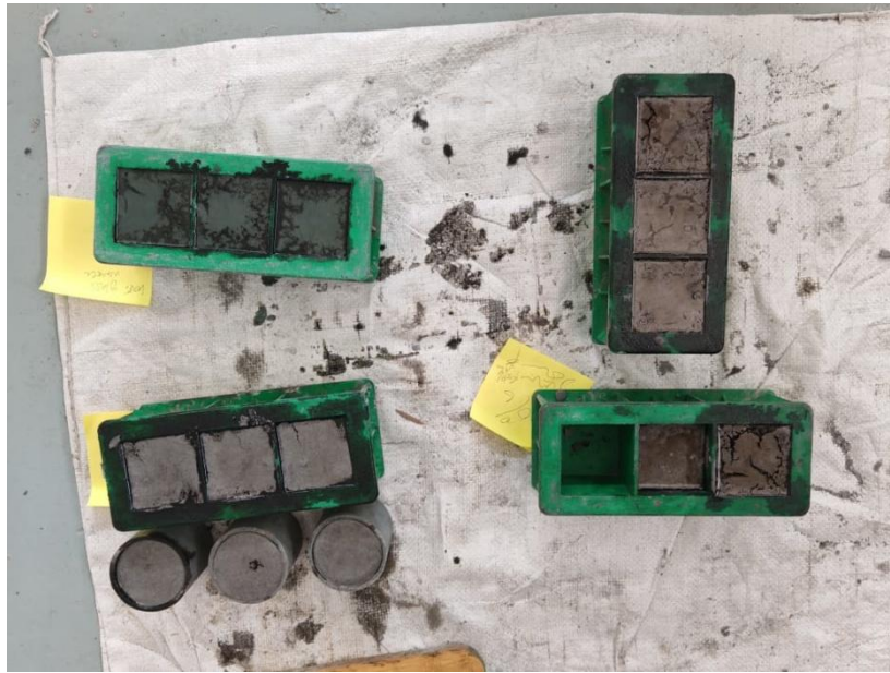
Figure 3.7: Moulding Process for Geopolymer
