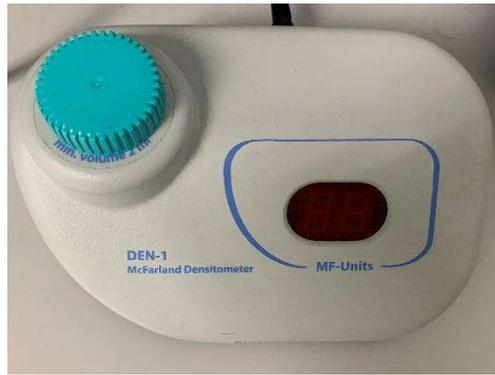
Figure 6. Densitometer for measuring cell density.
