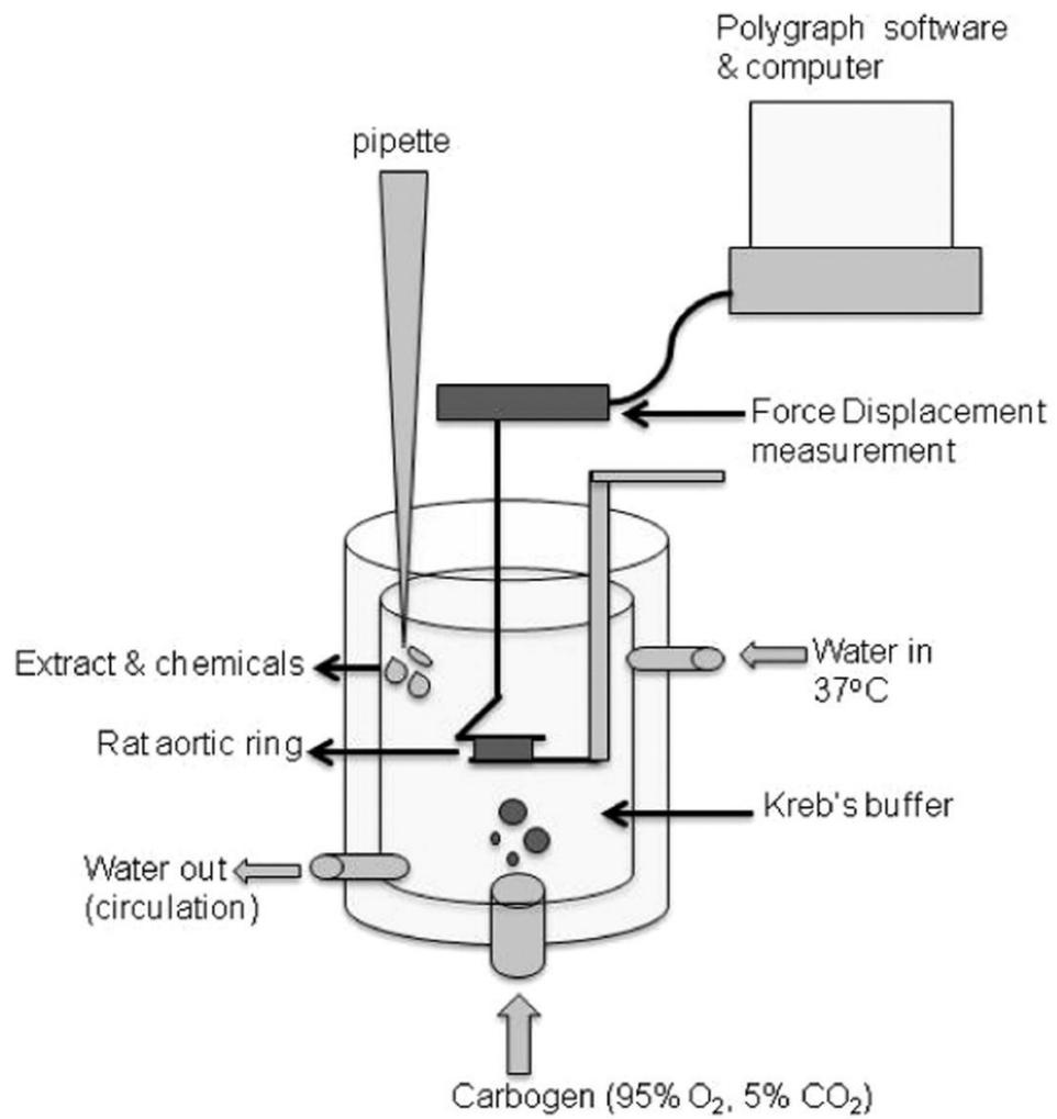
Figure 2.3: Schematic set-up of an organ bath (Shahlehi and Petalcorin, 2021).
