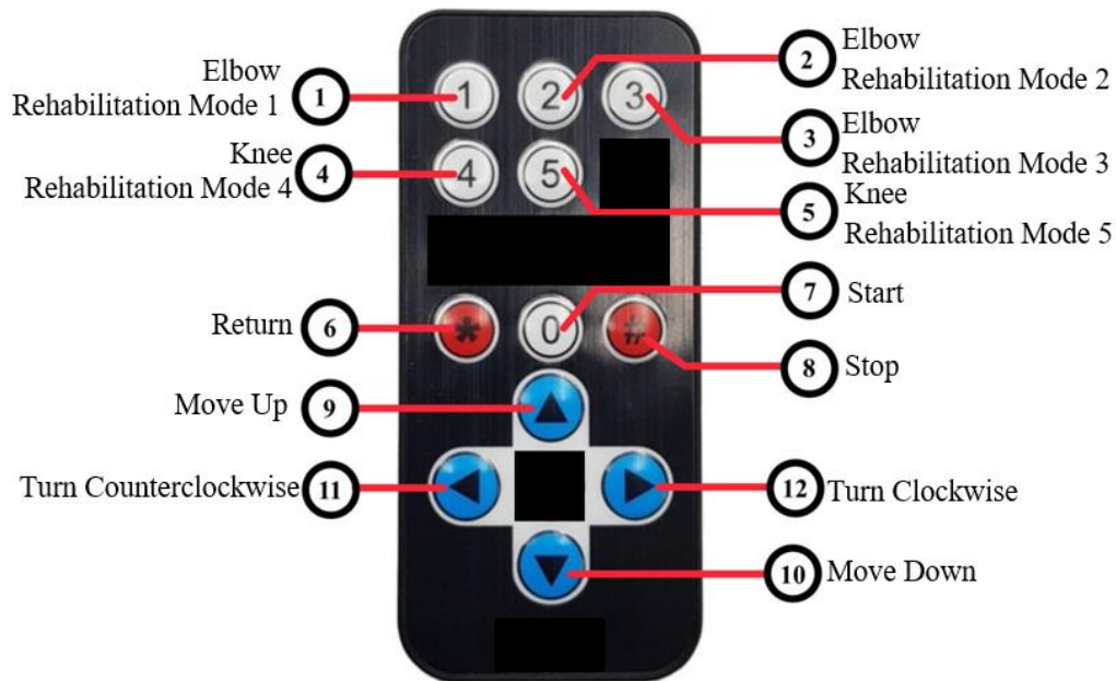
Figure 4.9: IR Remote Control – Button Layout and Labels.
