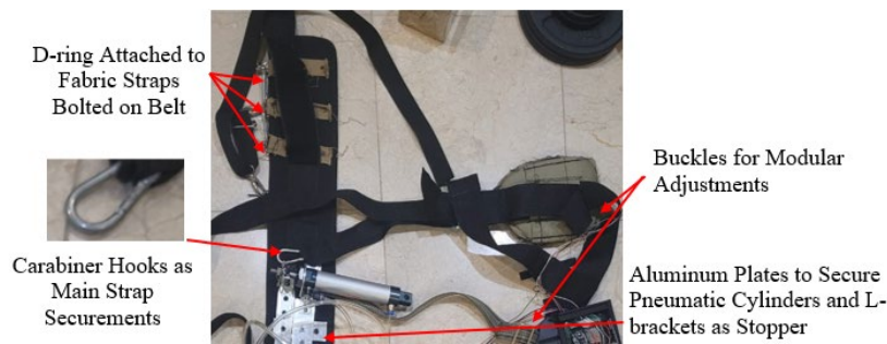
Figure 3.23: Fastening and Securement Strategies of the Prototype
