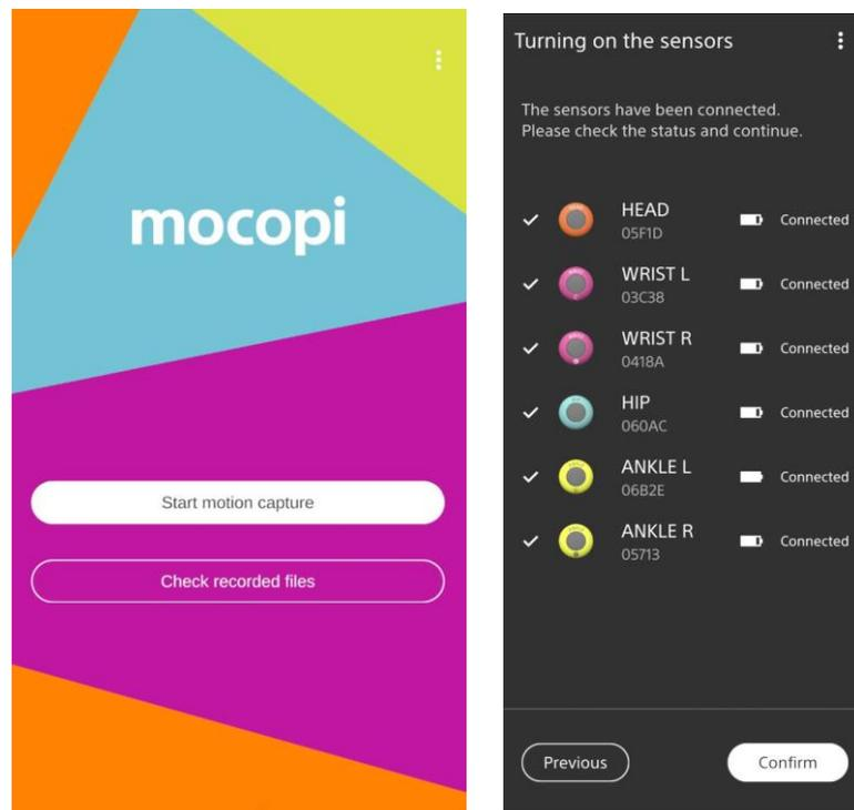
Six sensors connect wirelessly with the iPad-installed Mocopi app via Bluetooth
