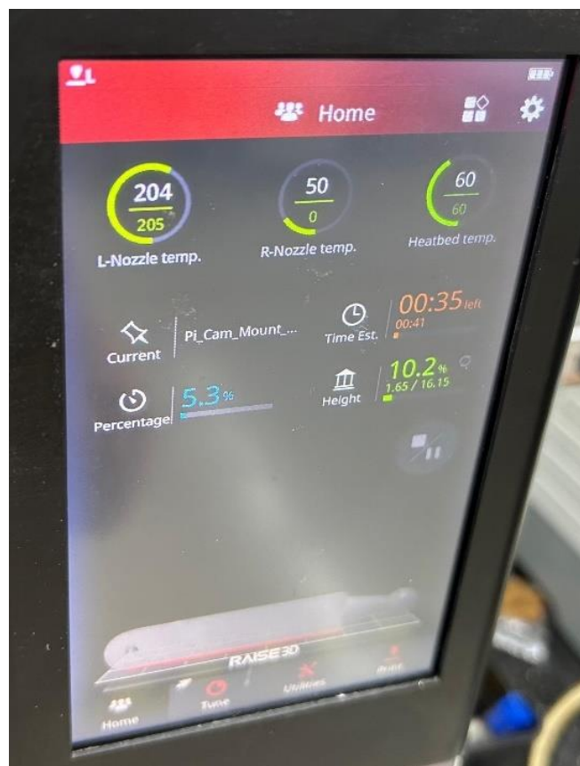
Figure 4.2: 3D Printer Home Setting for Raspberry Pi Camera Enclosure.
