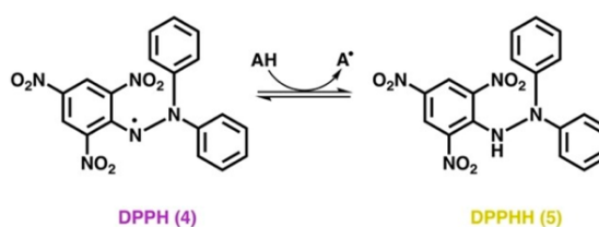
Figure 2.8: The working principle of DPPH assay (Higgins et al. , 2021).
