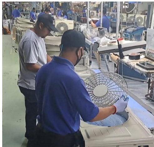
Figure 3.5: The assembly line workers are assembling air conditioner parts
