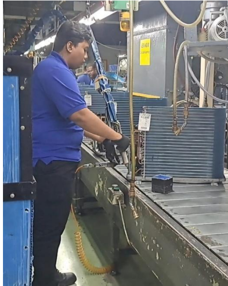
Figure 3.4: The assembly line worker is doing the leak testing for the refrigerant gases
