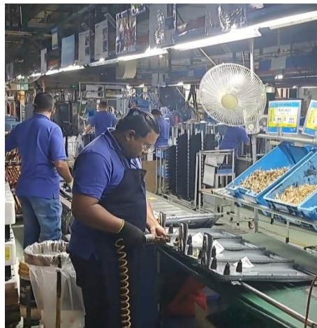
Figure 3.3: The assembly line worker is screwing the air conditioner parts
