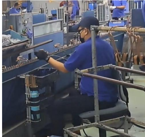
Figure 3.2: The assembly line worker is welding pipes for the air conditioner
