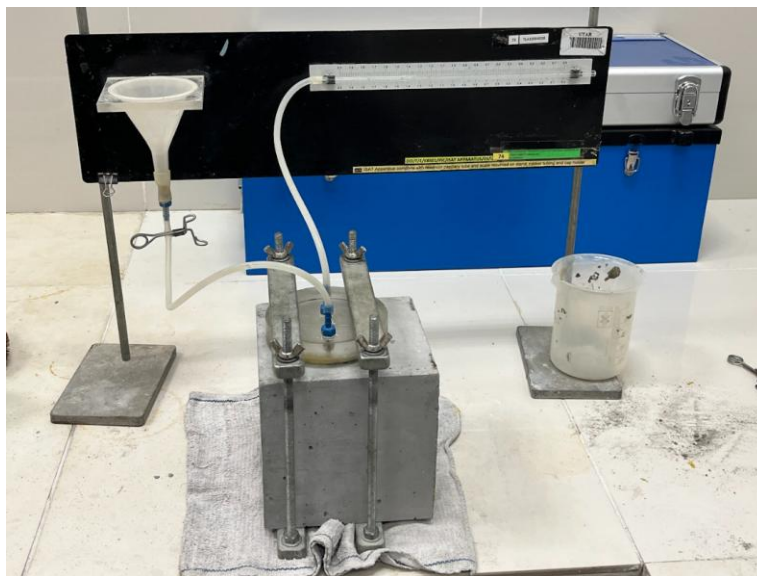
Figure 3.19: Setup of ISAT.
