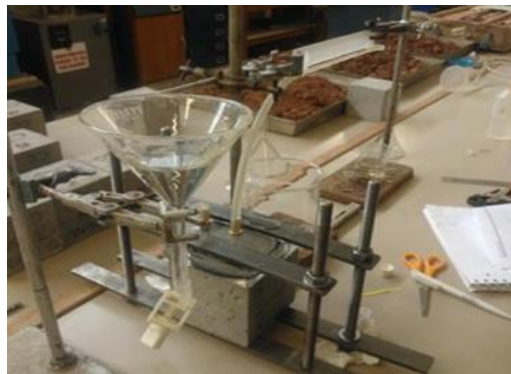
Figure 2.38: ISAT Instrument Setup (Balakrishna et al., 2018).
