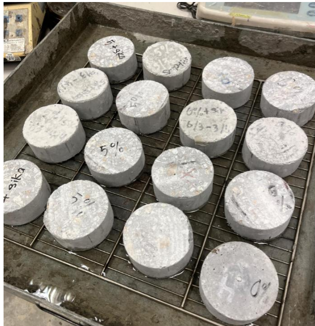
Figure 3.20: Setup of Sorptivity Test.
