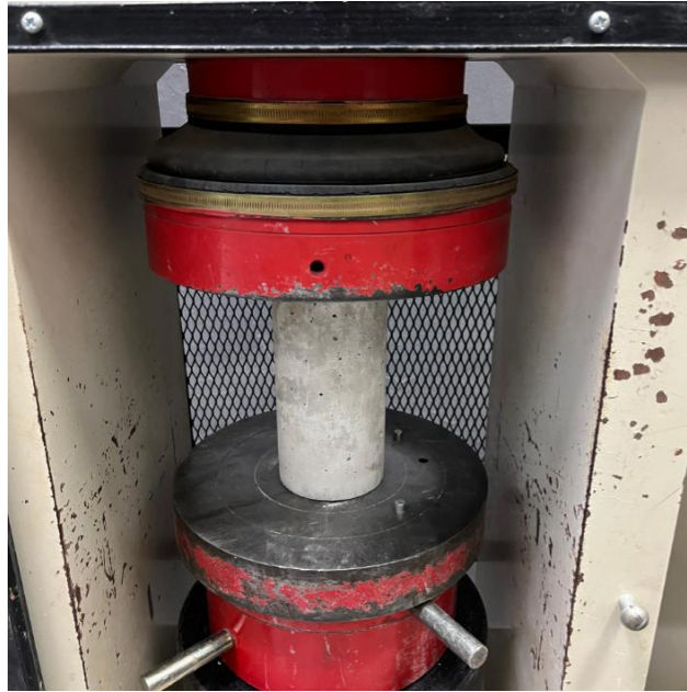
Figure 3.17: Setup of Compressive Strength Test.
