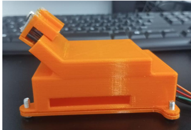
Figure 4.13 3D-Printed Raspberry Pi Case
