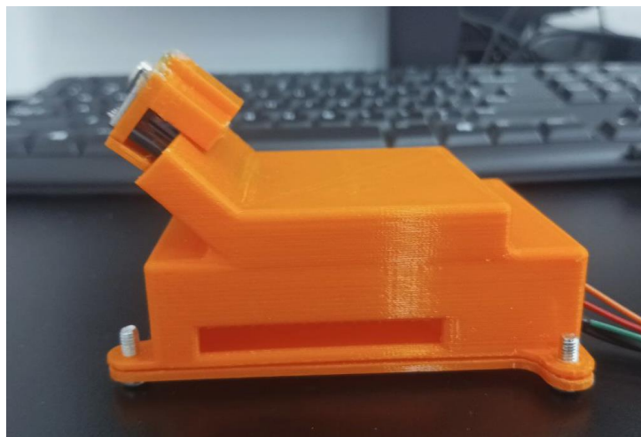
Figure 4.6 3D-printed Raspberry Pi Case
