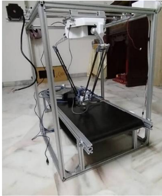
Figure 3.4: Assembly of Conveyor Belt and Frame of Delta X Robot Arm
