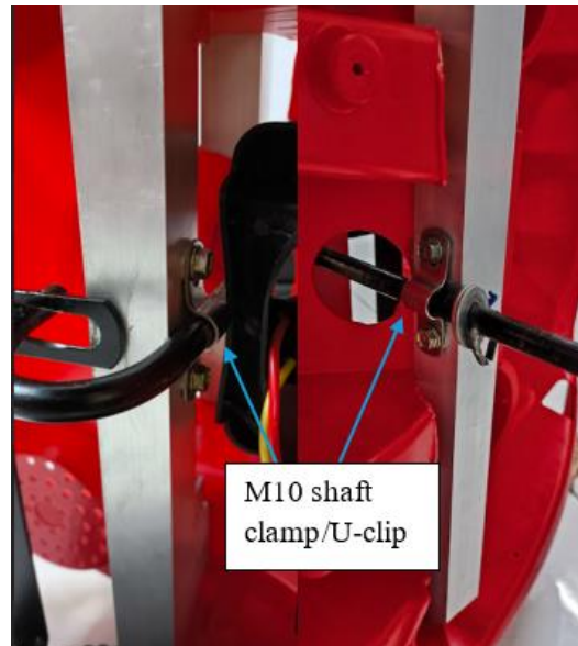
Figure 3.36: Steering column holding method.
