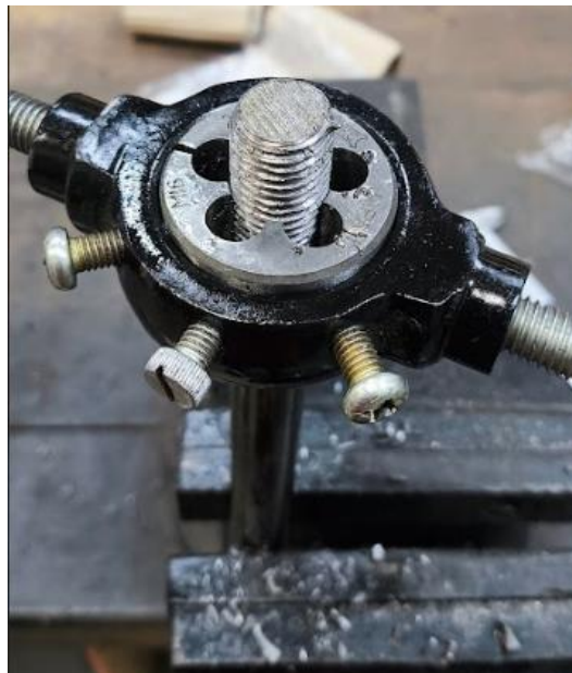
Figure 3.11: M16 \times 2.0 with 30 mm length thread.
