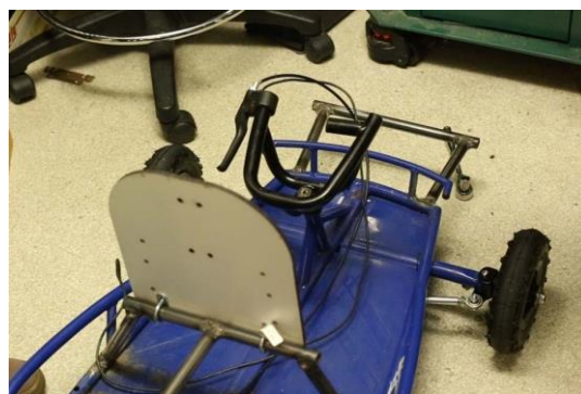
Figure 2.5: Finished electric ride-on-car setup without car body (Wu, 2016c).
