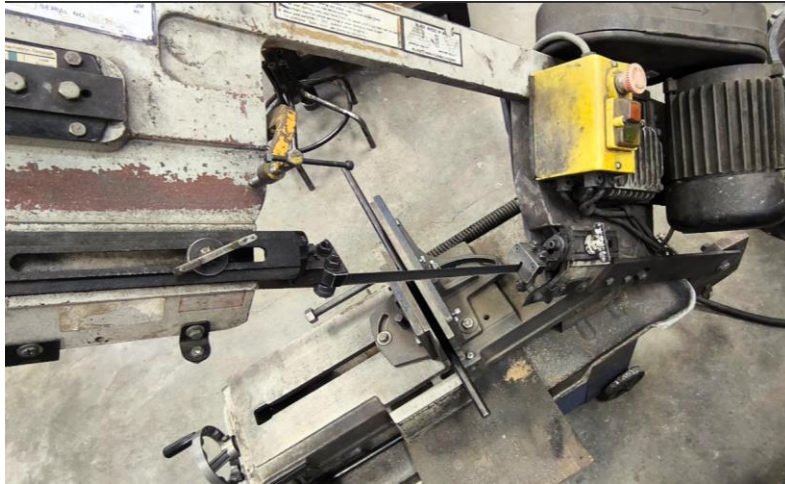
Figure 3.9: Cutting the 16 mm diameter shaft into length of 600 mm.
