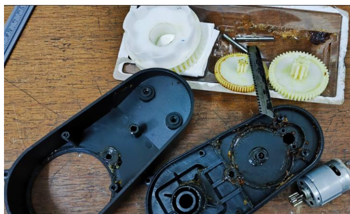
Figure 3.49: Separation of gearbox internal part.
