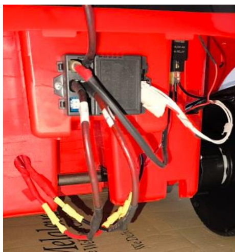
Figure 3.69: Upgraded motor controller.
