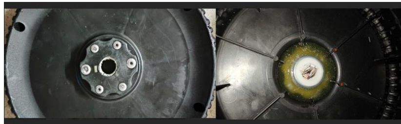
Figure 3.21: Rivet process and epoxy glue filling process of the inner wheel housing.
