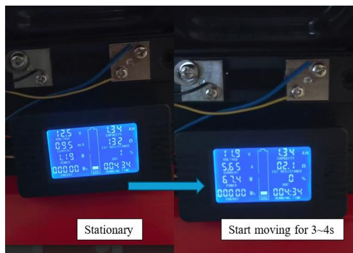
Figure 4.19: Power reading when the car starts to move for 3 to 4 second.
