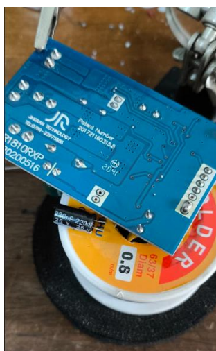
Figure 3.67: Removing original 25 V capacitor.
