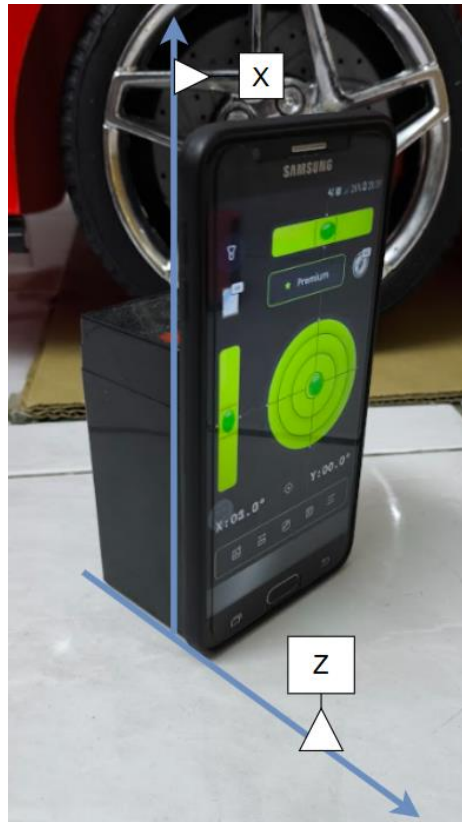
Figure 3.45: Measurement setup for wheel camber angle.
