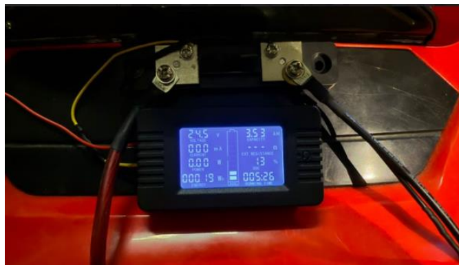
Figure 4.35: Power consumption of the modified ride-on-car after driving for 5 laps.
