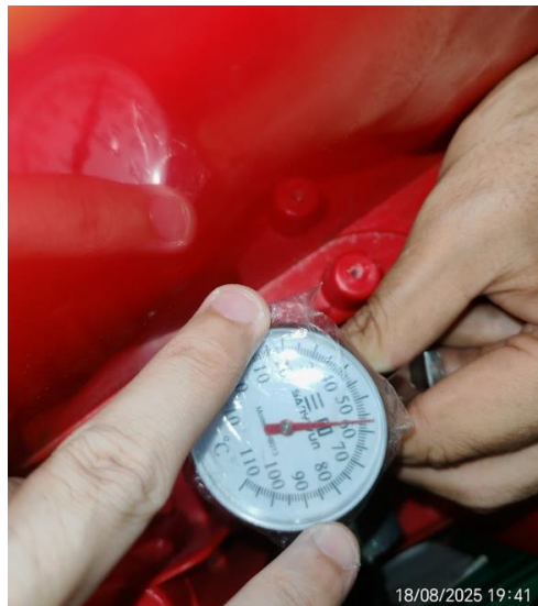
Figure 4.37: Motor temperature measurement after the second test.
