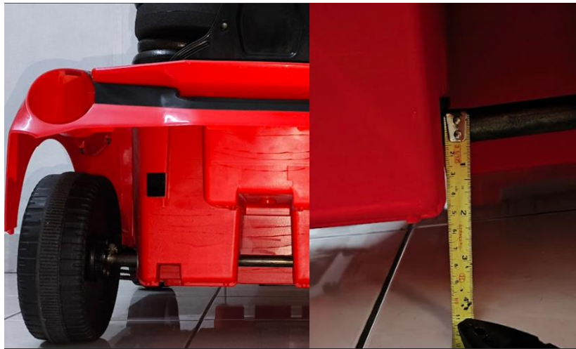
Figure 4.10: Result for shaft deflection after changing to 16 mm shaft (115 mm from datum).
