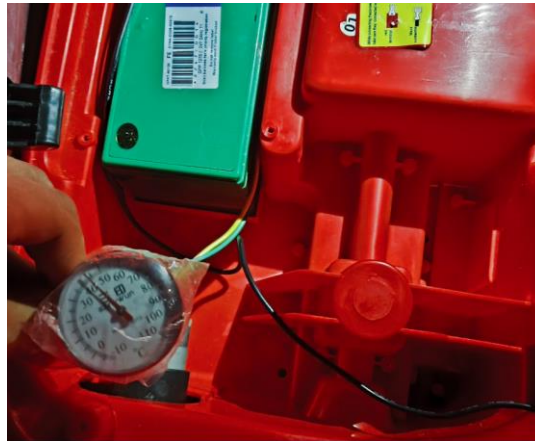
Figure 4.28: Motor temperature measurement after the first test.
