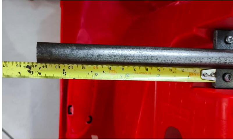
Figure 3.40: Measuring distance from the end of the shaft to cover plate.
