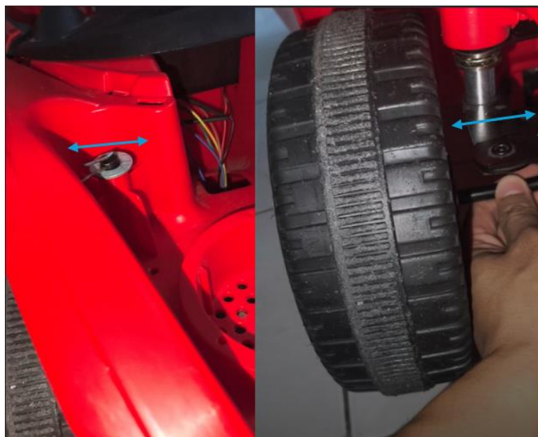
Figure 4.1: Movement (free play) of turning rod and wheel assembly due to excessive camber increment.
