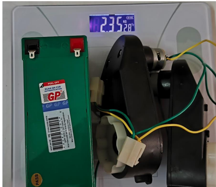
Figure A.9: Stock 12 V motor gearbox weight
