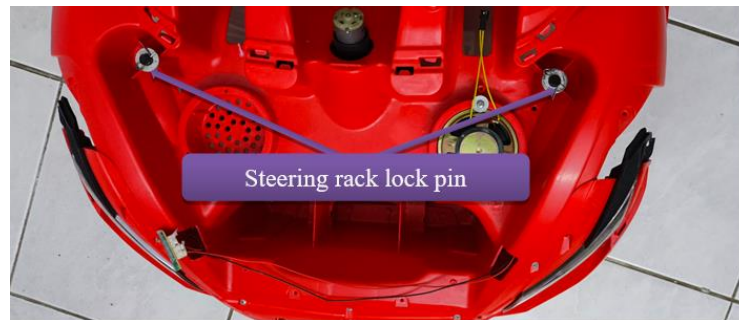
Figure 3.34: Steering linkage lock pin.
