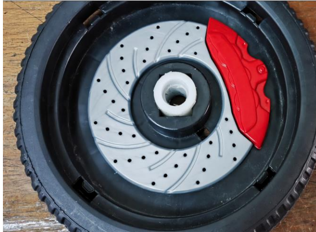
Figure 3.17: Nylon bushing for frontside of wheel.
