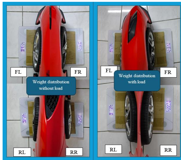
Figure 4.12: Weight distribution diagram after suspension reinforcement.
