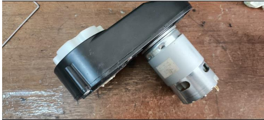
Figure 3.56: RS895 motor-gearbox set with first gear delete.
