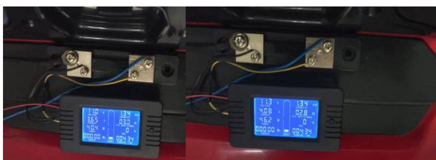
Figure 4.20: Power reading when the car reached constant speed.
