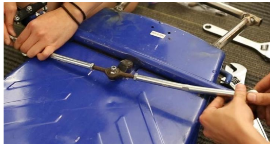
Figure 2.4: Steering linkage setup (Wu, 2016c).
