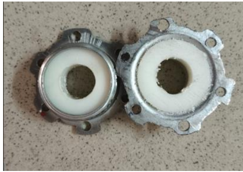
Figure 3.20: Test fit the inner wheel housing with nylon bushing.
