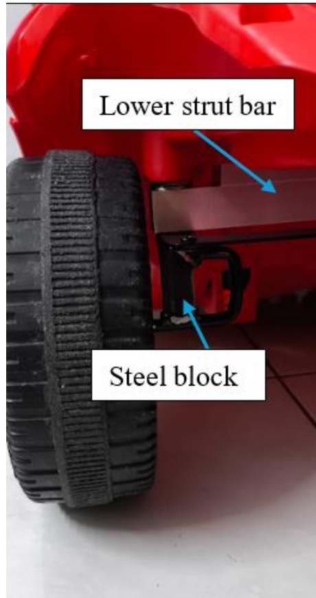
Figure 4.2: Camber change under load after reinforced steering assembly.
