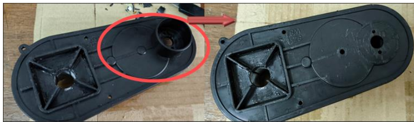
Figure 3.52: Fabrication of the new motor mounting location.
