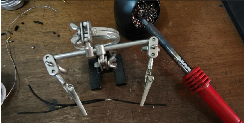
Figure 3.59: Wiring harness fabrication process.
