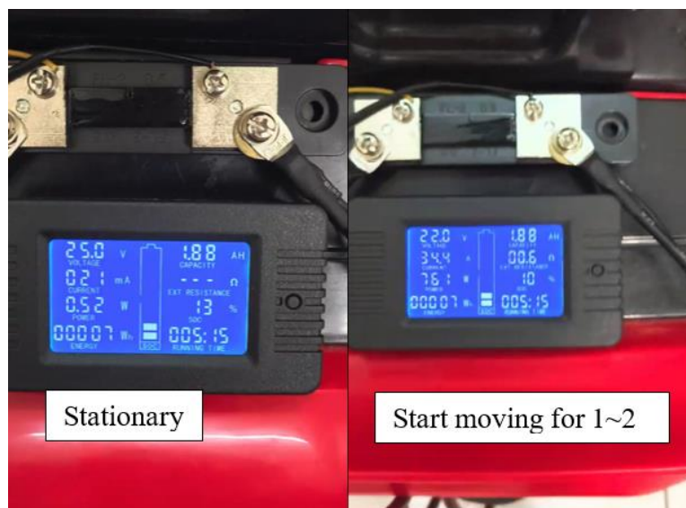
Figure 4.31: Peak power reading from stationary condition.
