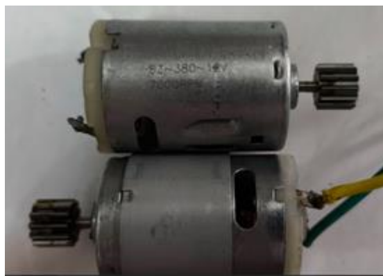
Figure 3.46: DC traction motor (upper one is steering remote motor).
