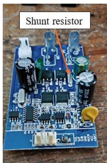
Figure 3.68: Soldering 50V capacitor and shunt resistor.
