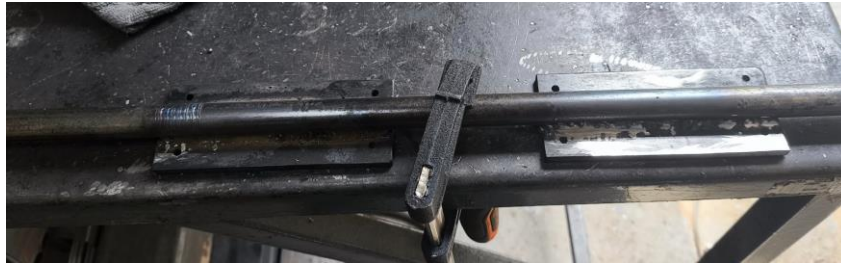
Figure 3.42: Fully welded rear shaft assembly.
