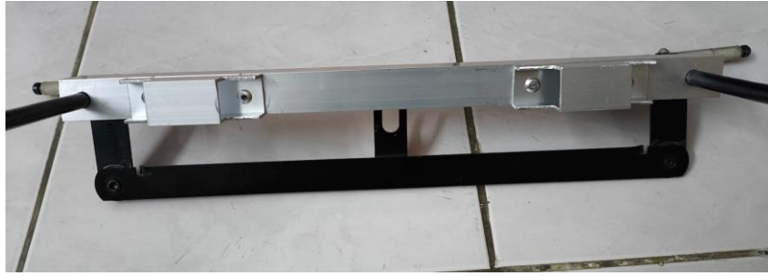
Figure 3.33: Lower half steering linkage reinforce bar.
