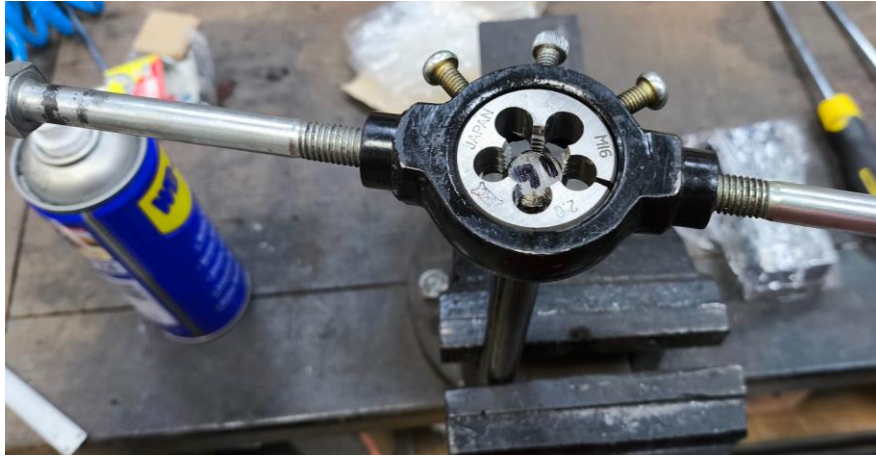
Figure 3.10: Process to make M16 \times 2.0 with 30 mm length.
