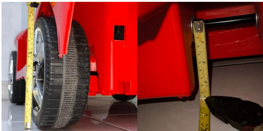
Figure 4.9: Result for shaft deflection from unload to loaded with 80 kg weight.
