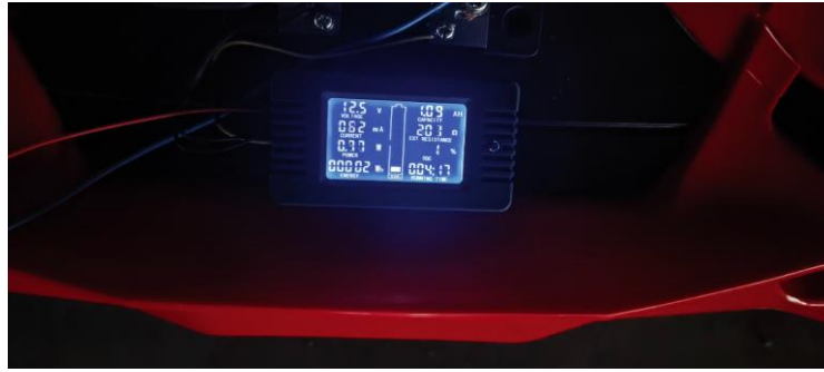
Figure 4.26: Power consumption of the ride-on-car after 5 laps.
