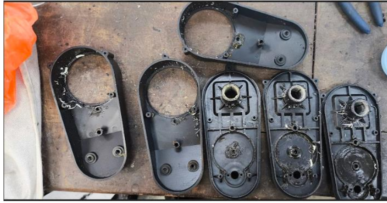
Figure 3.51: Outcome of drilled output gear holes.
