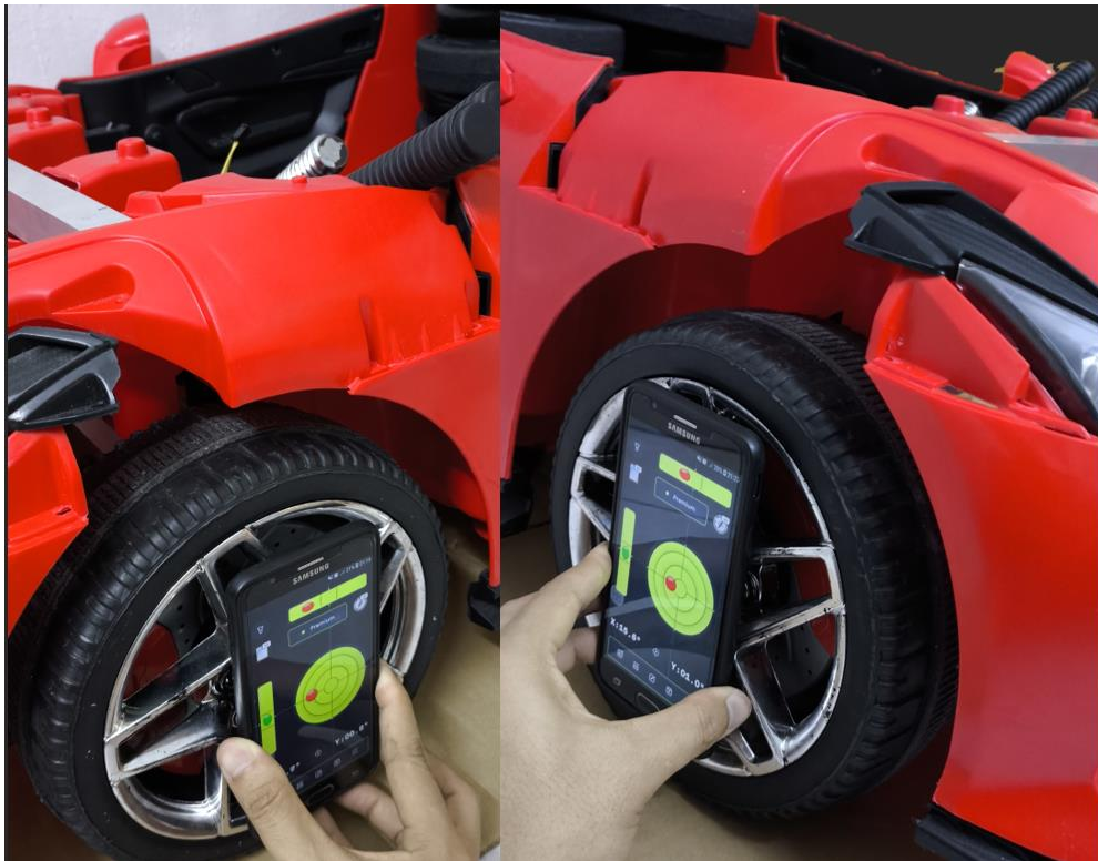
Figure 4.6: Wheel camber measurements with aluminium strut bar (left and right wheel).
