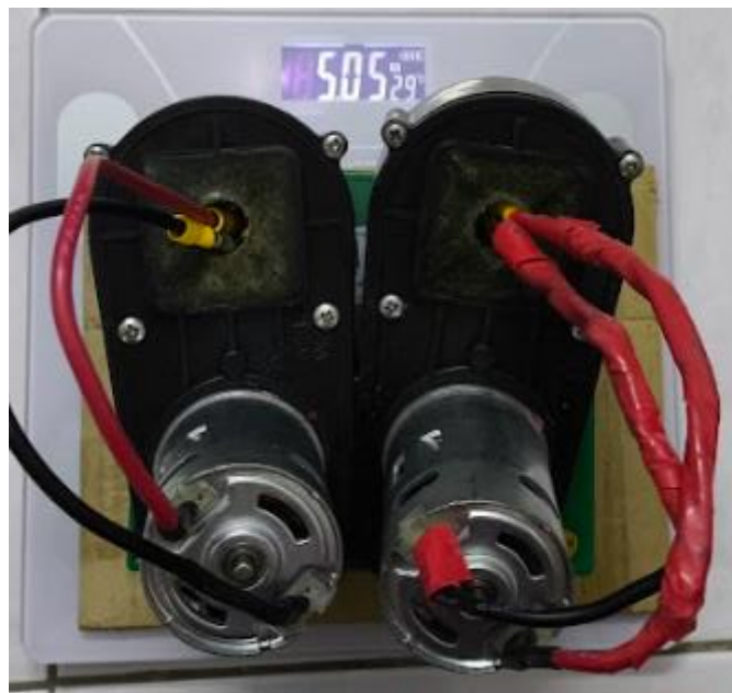
Figure A.10: Upgraded 24 V motor gearbox weight
