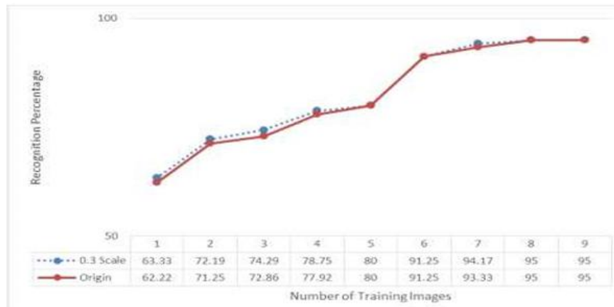
Figure 2.2.2.4 Recognition Rate After Resized by Scale 0.3
