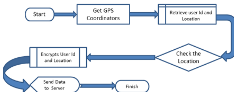
Figure 2.1.2.2 Flows of operation for mobile application
