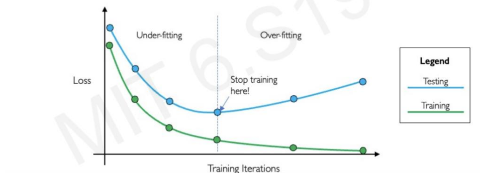
Figure 4.1.4 Early Stopping to minimize overfitting
