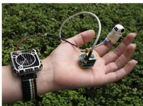
Figure 2.2.3 (g): Pulse oximeter powered by watch-style thermoelectric generator (Ghomian and Mehraeen, 2019).
