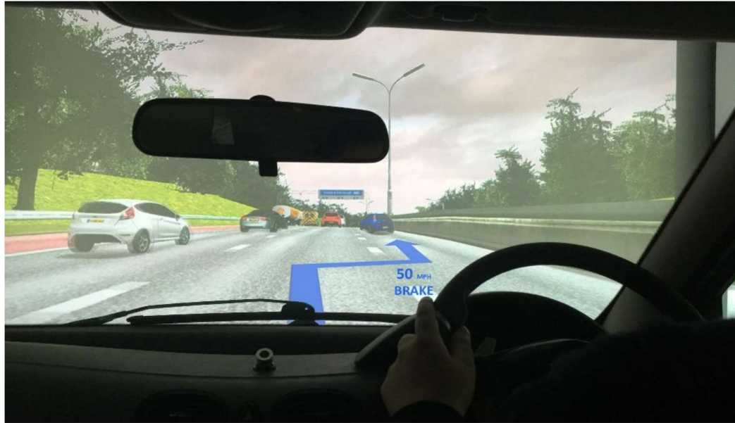
Figure 2.33: Intelligent Collision Avoidance and Manoeuvring System [82]
