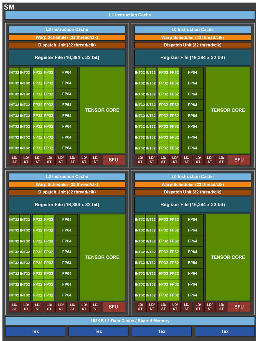
Figure 3.1: Nvidia's Ampere SM Architecture
