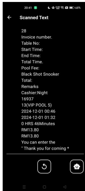
Figure 5.2.3.2 Scanned text using google ml kit text recognition
