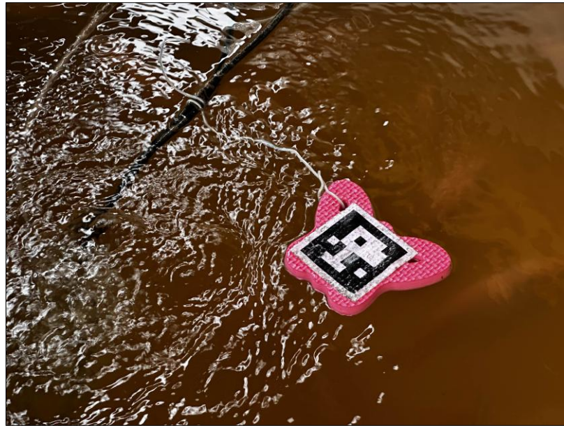
Figure 5.1.2. Printed ArUco marker affixed to float placed on water surface
