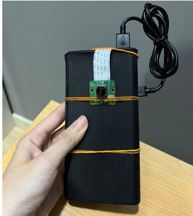
Figure 6.9 Pi Camera Attached to a Power Bank
