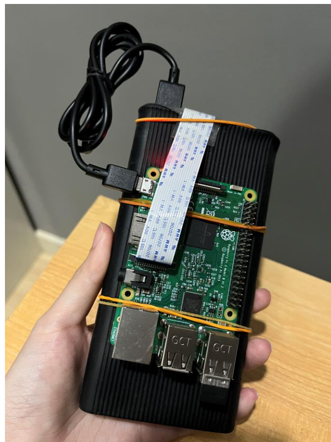
Figure 6.10 Raspberry Pi Attached to a Power Bank
