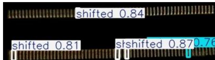
Figure 6.2.3 Defect Pin Detection Model (Generate Case)
