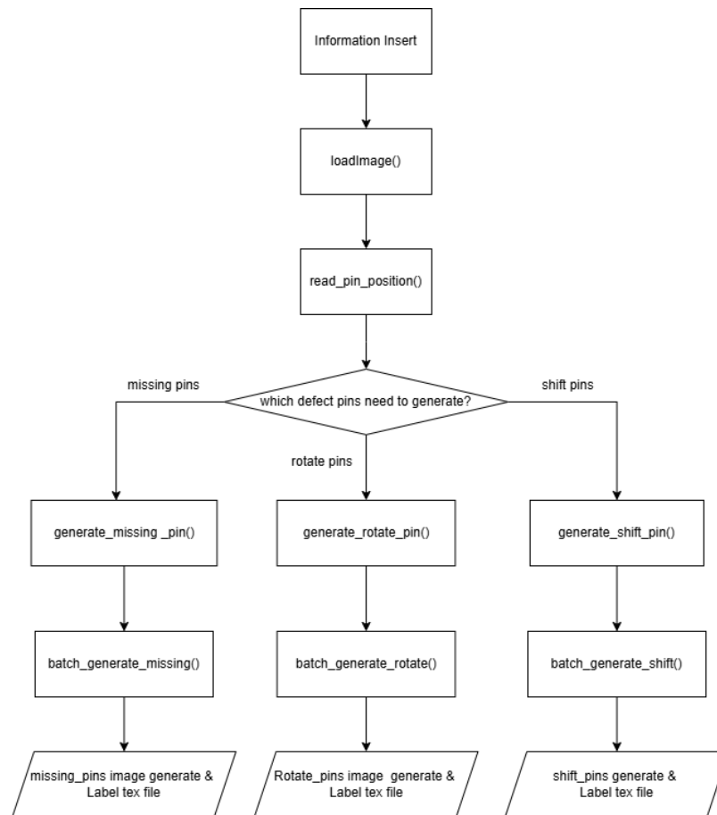
Figure 4.2.7 Defect Pins Generation Workflow
