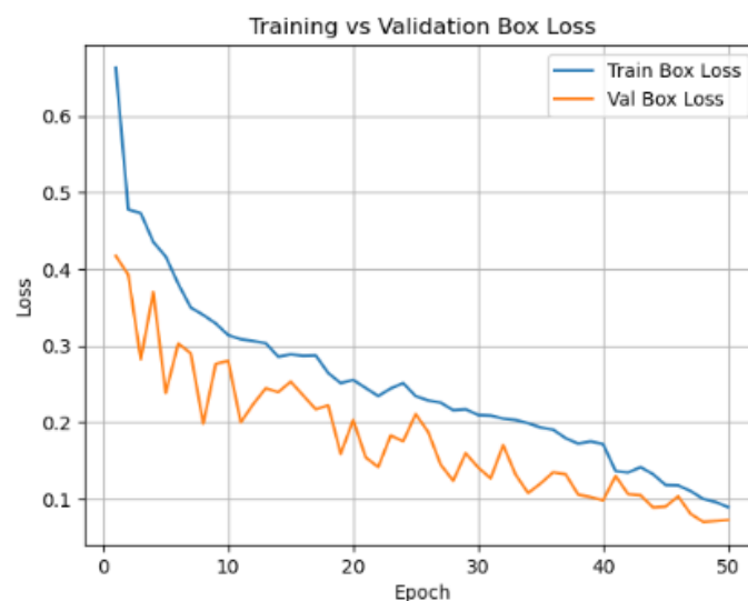
Figure 6.1.4 Region Detection V2 - Training vs Validation Box Loss Curve
