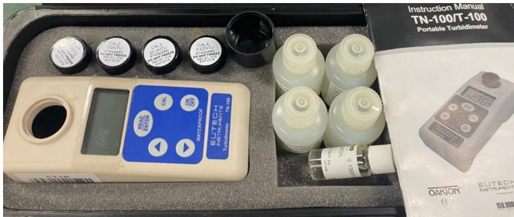
Figure 3.11: Waterproof TN 100 Waterproof Turbidimeter.
