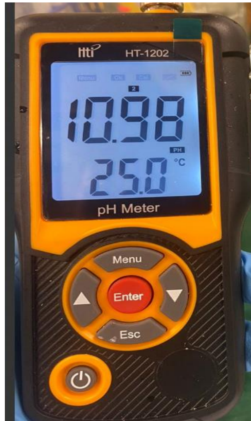
Figure 3.14: HT-1202 PH Meter.
