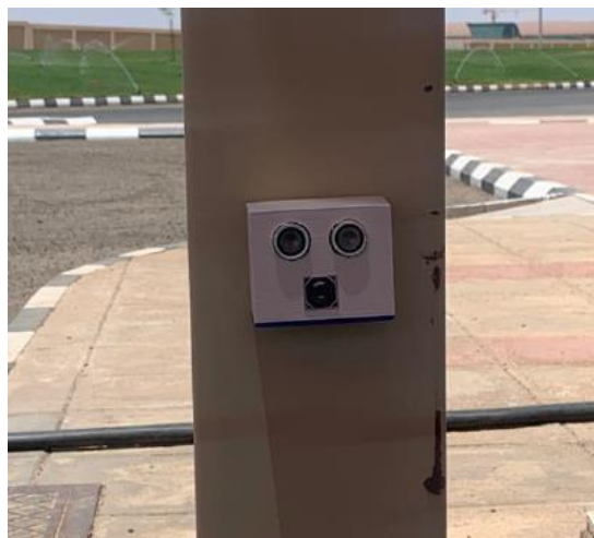
Figure 2.13: The Monitoring Unit Consists of Range Finder Sensor and Camera (Elfaki et al. , 2023)
