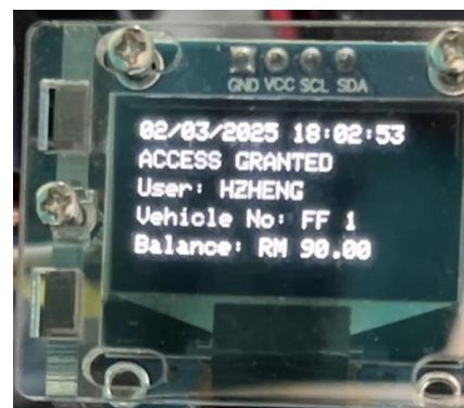
Figure 4.51: OLED Display Showing Access Authorized Messages
