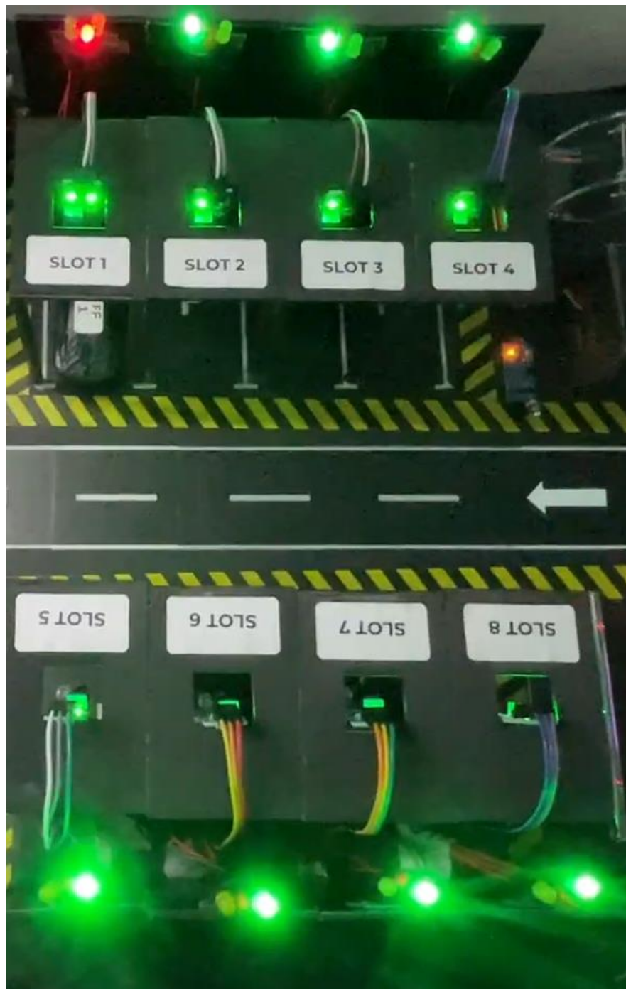
Figure 4.61: Slot 1 Red LED Lights Up After the User Parks in the Reserved Slot
