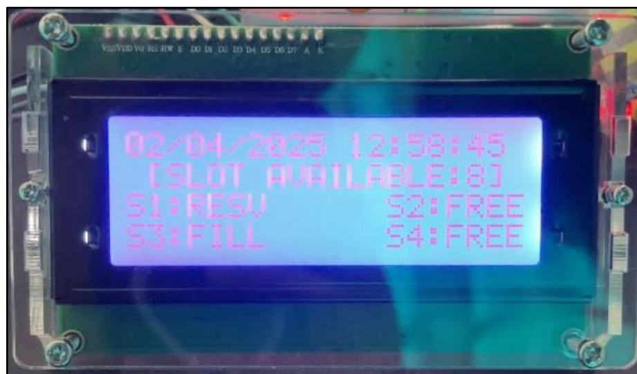
Figure 4.45: LCD Display Showing the Current Time, Number of Available Parking Slots, and the Status of Each Slot
