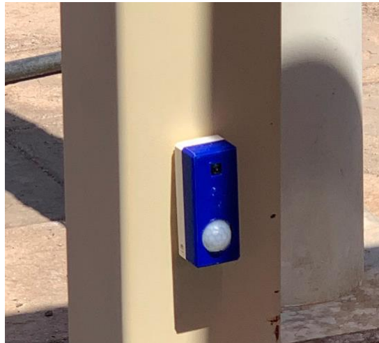
Figure 2.12: The Monitoring Unit Consists of Motion Sensor and Camera (Elfaki et al. , 2023)
