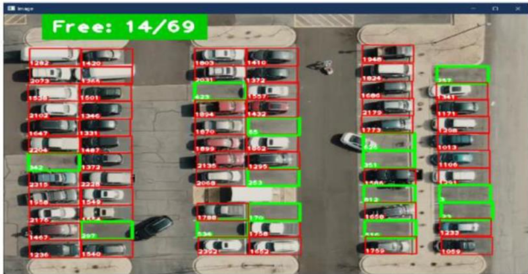
Figure 2.11: Vacant Slot Detection (Lincy et al. , 2024)
