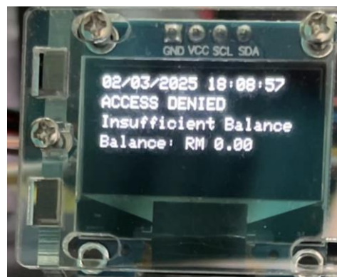
Figure 4.53: OLED Display Showing Insufficient Balance Messages
