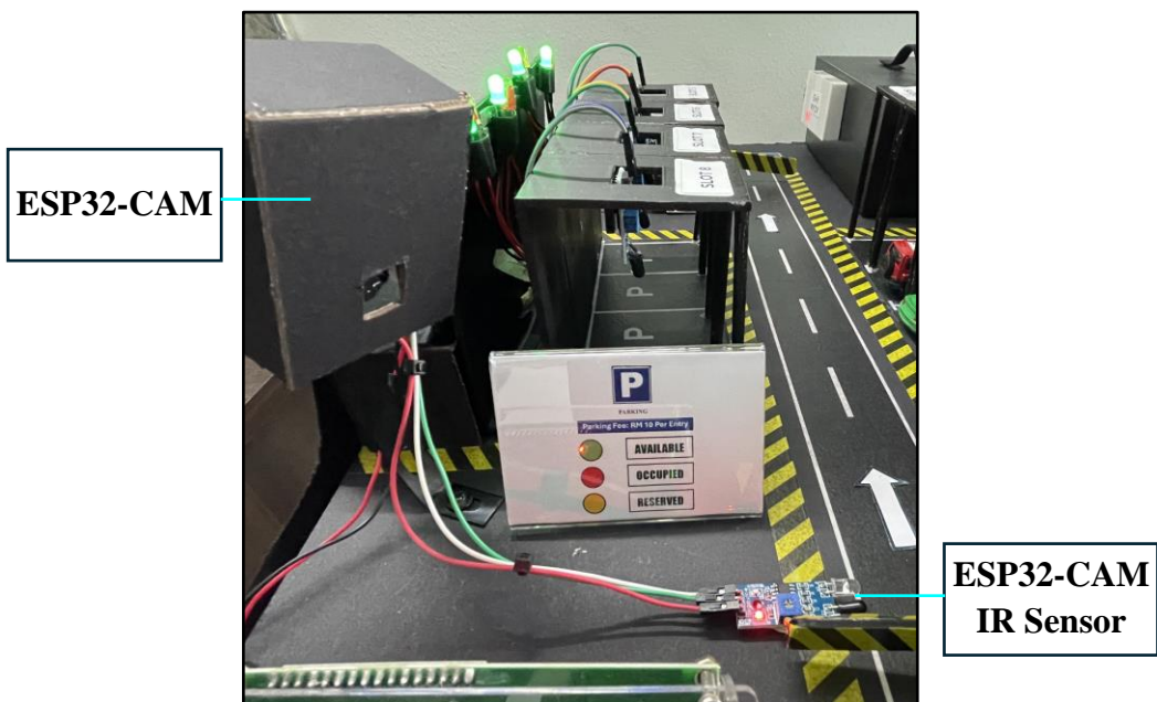
Figure 4.46: ESP32-CAM and IR Sensor Image-Capturing System at the Entrance
