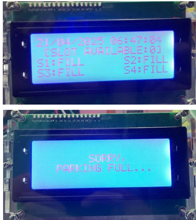
Figure 4.59: LCD Messages when All Parking Slots are Occupied (Parking Full)
