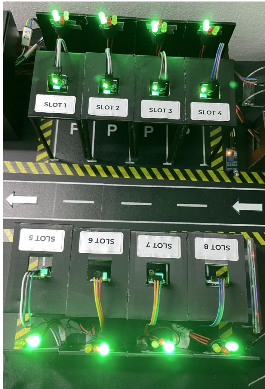
Figure 4.62: Slot 1 Green LED Lights Up After Reservation Time Passes
