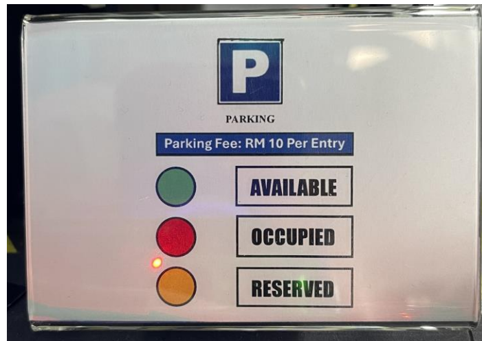
Figure 4.44: Entrance Display Board Showing Parking Fees and LED Light Meanings
