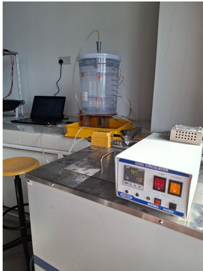
Figure 3.35: Testing Setup With The Water Bath (right), Prototype Tank (center) and Computer (left) For Data Logging
