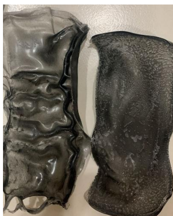
Figure 5-1: Right Handside is the One Used Silicon Mold and Left Handside is the One Used Metal Plate
