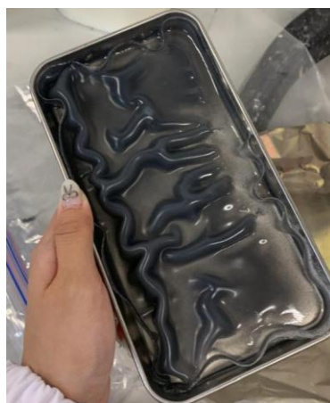
Figure 5-2: The Wrinkle Appearance of the Failed Example
