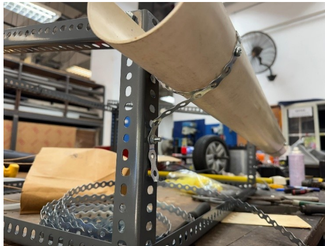
Figure 3-6: Attached Gutter on Frame
