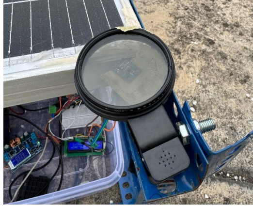
Figure 3-13: Solar Irradiance Data Logger
