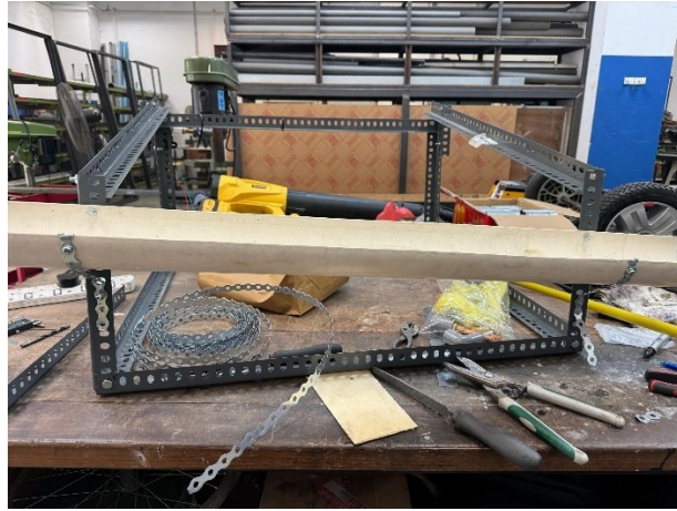
Figure 3-5: Gutter System for Water Flow
