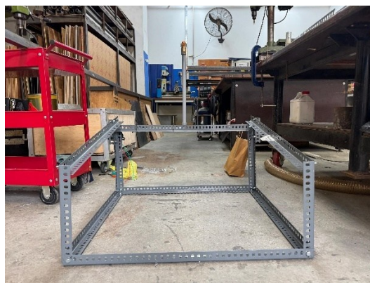
Figure 3-4: Frame Assembly using Perforated Steel Members
