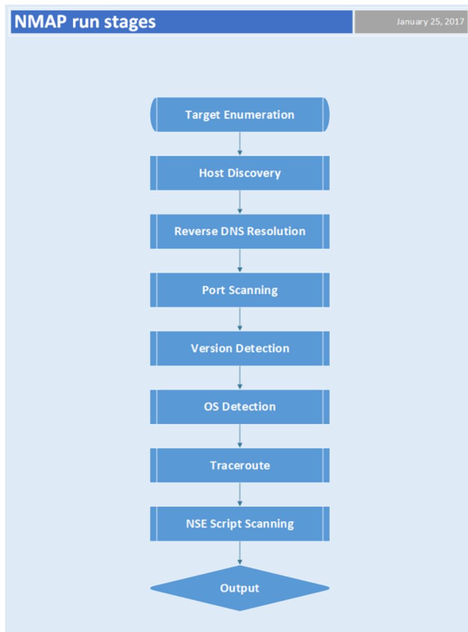
Figure 2.1 Nmap scanning workflow
