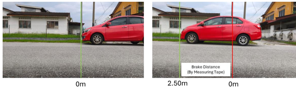
Figure 6.6 Physical measurement of emergency braking distance
