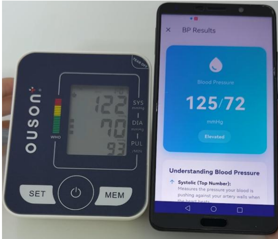
Figure 6.2.1.3 Result on Validating XGBoost BP Estimation Model using Ouson arm-type electronic BP monitor.
