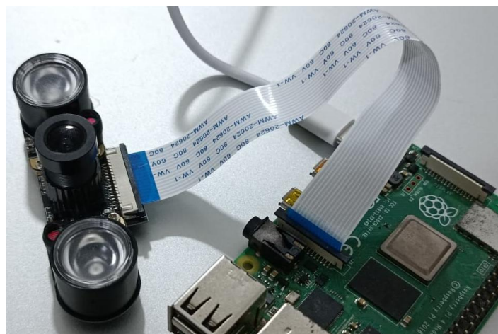
Figure 5-2: Camera Module Connected to Raspberry Pi 4
