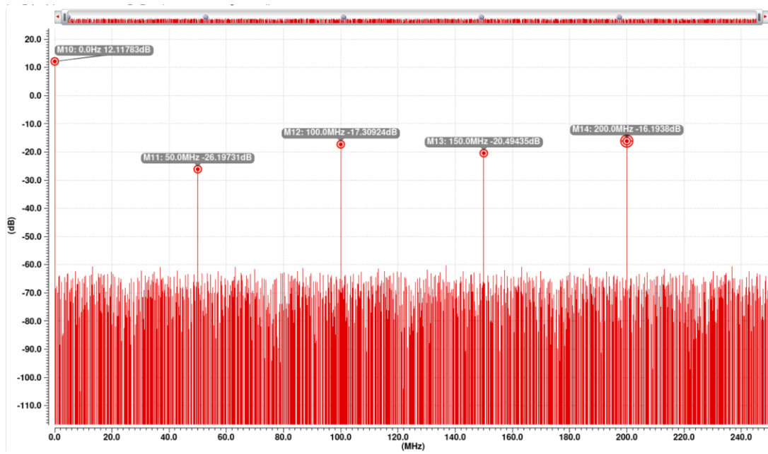
Figure 4.35: FFT Result of Charge Pump Output Signal with V_{DD} at 2.5 V
