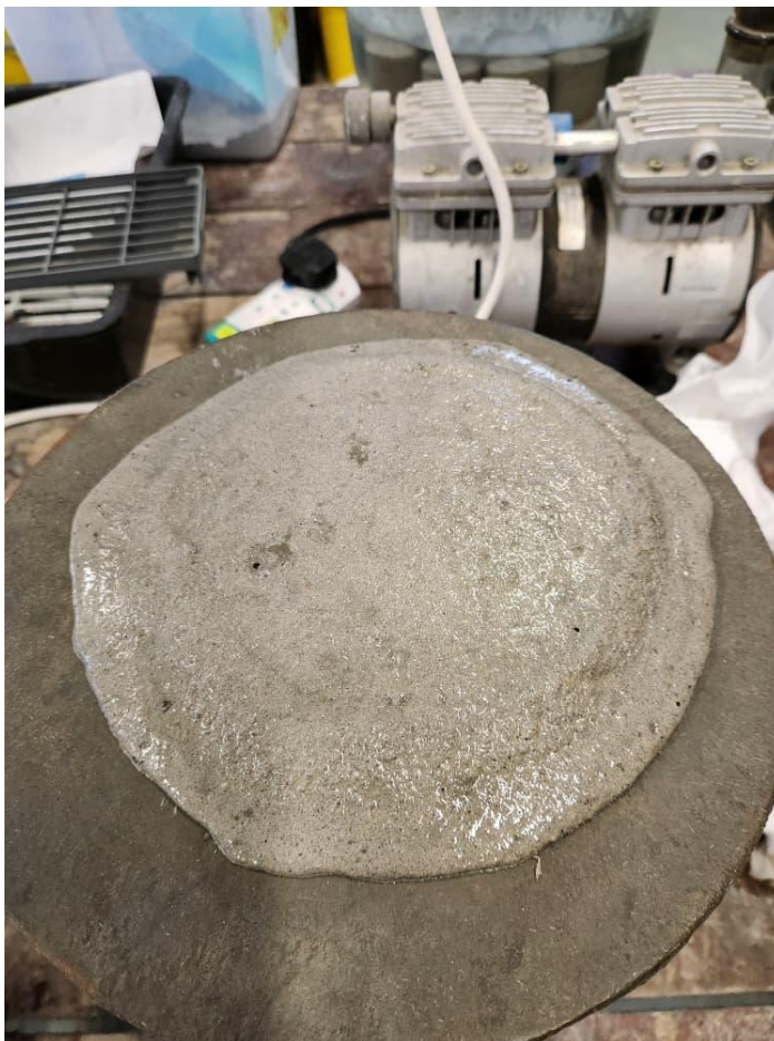
Appendix A: C10-P22.5G67.5 Flow Test
