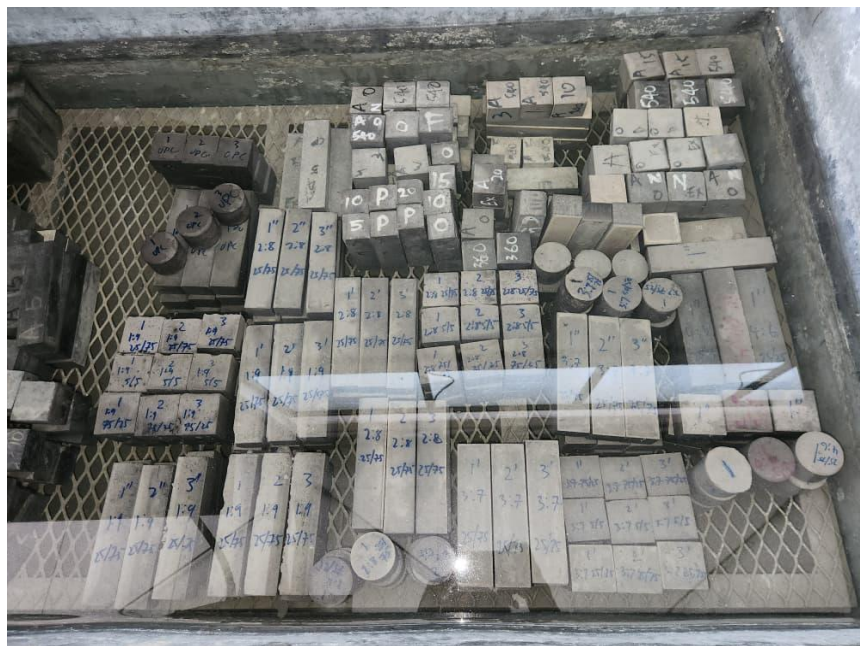
Figure 3.13: Water Tank for Curing
