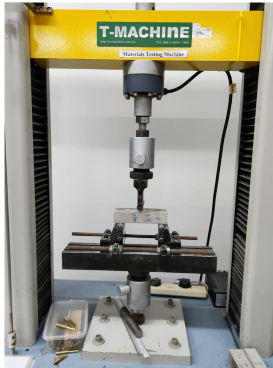
Figure 3.16: Flexural Strength Test Machine
