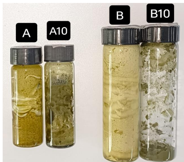
Figure 4.3: Extracts obtained using pure CO 2 SCE and 10%-ethanol-assisted extraction. A: SCE of younger Eucalyptus ; A10: Ethanol-assisted SCE of younger Eucalyptus ; B: SCE of older Eucalyptus ; B10: Ethanol-assisted SCE of older Eucalyptus .
