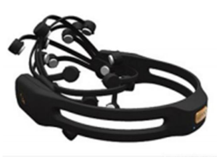
Figure 3.9: Emotiv EPOC EEG wireless headset (Emotiv Systems Inc., San Francisco, CA, USA) (Kawala-Janik, et al., 2013)
